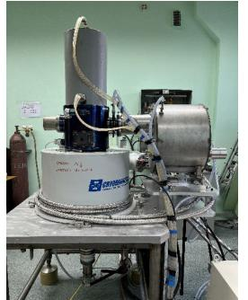
Around 2016 one of the gyrotrons experienced rapid cathode degradation, was repaired, but eventually was replaced with a new triode 800 kW gyrotron.
