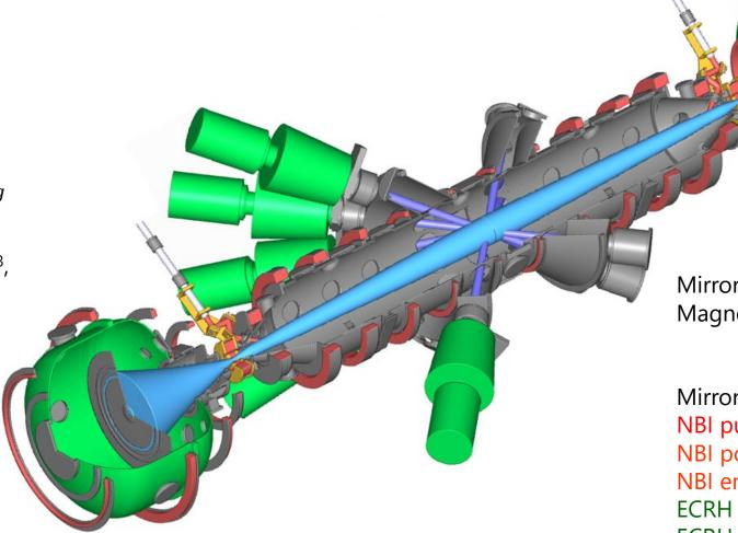
7 m Mirror-to-mirror Magnetic field: 0.35 T center mirrors 12 T Mirror ratio 35 5 ms NBI pulse duration **NBI** power 5 MW NBI energy 23 keV ECRH power 1.2 MW ECRH pulse duration 8 ms
