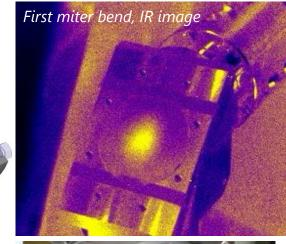
The was a short experimental test of planar resonant absorbers and the technique has a potential for time-resolved frequency-selective microwave power measurements.
