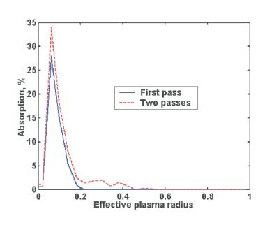
X2 absorption calculated with  $B_0$ =0.5T,  $n_{eo}$ =2.0 x10 $^{18}$ m $^{-3}$ ,  $T_{eo}$ =0.4keV
