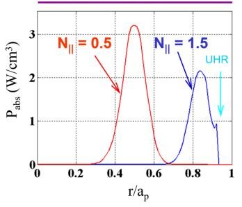
EBW absorption calculated with  $B_0=1T$ ,  $n_{eo}=1.2 \times 10^{19} \text{m}^{-3}$ ,  $T_{eo}=2 \text{keV}$
