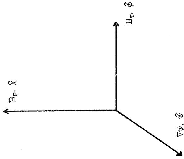
Fig. 3-1. Coordinate system used.  $\hat{\phi}$  and  $\hat{X}$  are tangent to the flux surface, in the toroidal and poloidal directions, respectively.  $\hat{\psi}$  is perpendicular to the flux surface.
