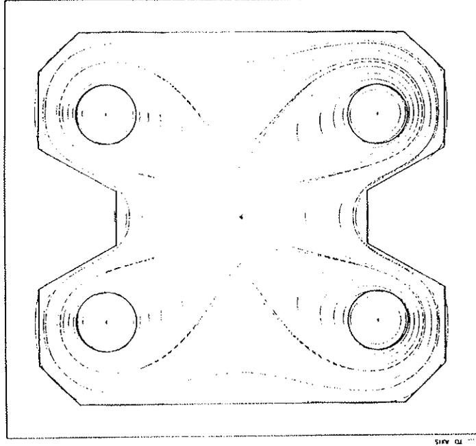
Fig. 2-2. Poloidal flux plot of octupole superimposed on outline of boundary conductors.
