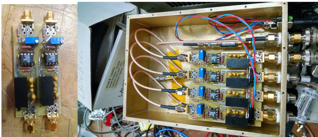
**Figure 3.15.** High speed diode power detector amplifier board (left), and 4 channel power detector module (right).
