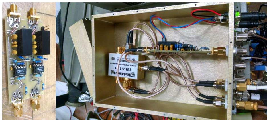
**Figure 3.23.** VVA driver board(left) and assembled VVA system (right).
