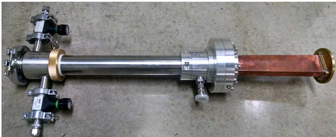
**Figure 3.2.** Cylindrical waveguide antenna. Leftmost component is a differentially pumped seal allowing the molybdenum antenna (center left) to slide and rotate without admitting gas to MST. Rectangular to cylindrical transition (rightmost) connects cylindrical pillbox window (center right) to the waveguide leading to the klystron tube.
