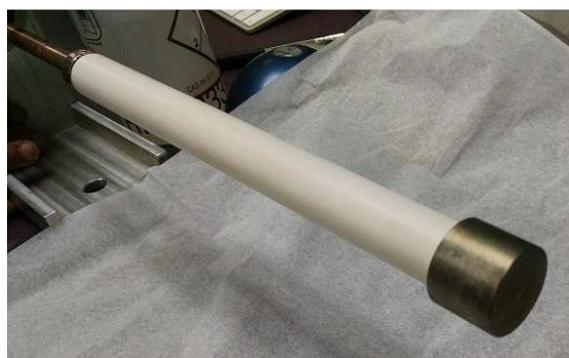
**Figure 3.45.** Target probe tip including a 25mm diameter, 25mm length molybdenum cylinder and boron nitride shield surrounding adjustable length copper rod.
