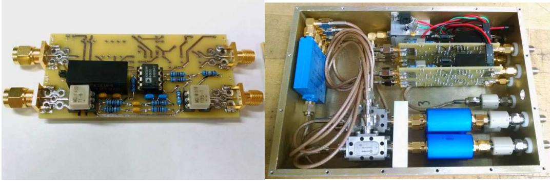
**Figure 3.13.** Phase detector amplifier board (left) with one of the two channels populated. Assembled 4 channel phase detector (right).
