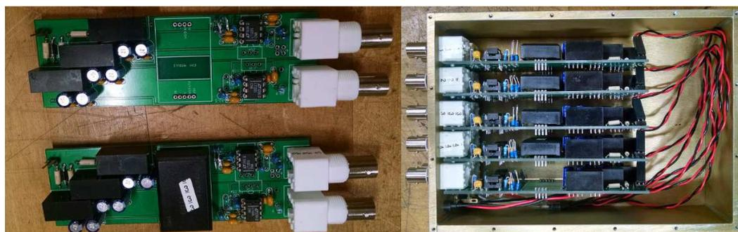
**Figure 3.8.** High speed isolation amplifier boards are shown on the left, boards mounted within an RF shielded enclosure are shown on the right.
