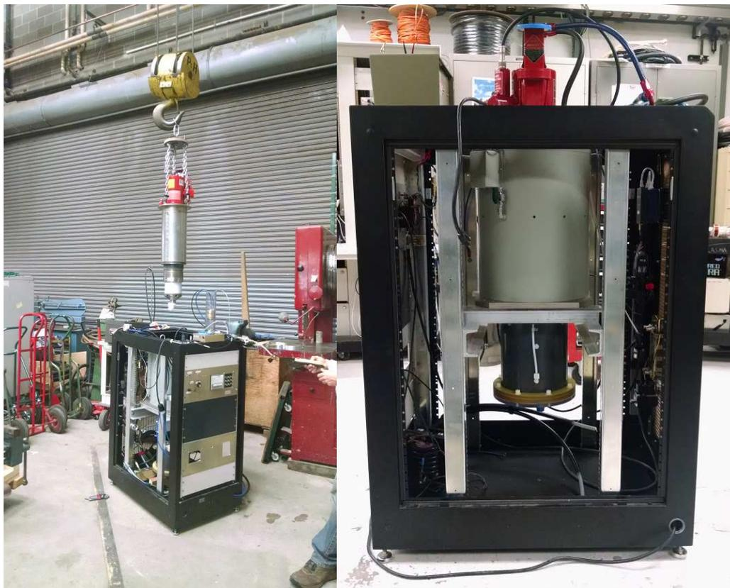
**Figure 3.1.** Klystron tube being lowered into magnet (left). Klystron in magnet assembly with cooling oil bath attached (right).
