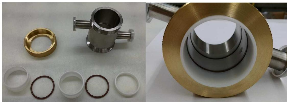
**Figure 3.3.** Differentially pumped sliding seal for cylindrical molybdenum antenna. Seal components (left) shows arrangement of o-rings and plastic spacers that stack within the stainless case. Assembled seal (right), shows pumping port located between the two o-rings. Plastic spacers provide ground loop isolation by insulating antenna from the shell of MST.
