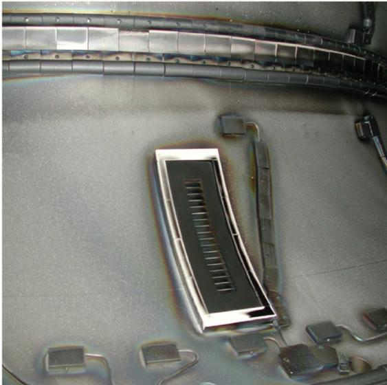
**Figure 3.46.** Lower hybrid antenna assembly including boron nitride limiter(white) and molybdenum interdigital straps(horizontal bars in center). Picture courtesy of John Goetz.
