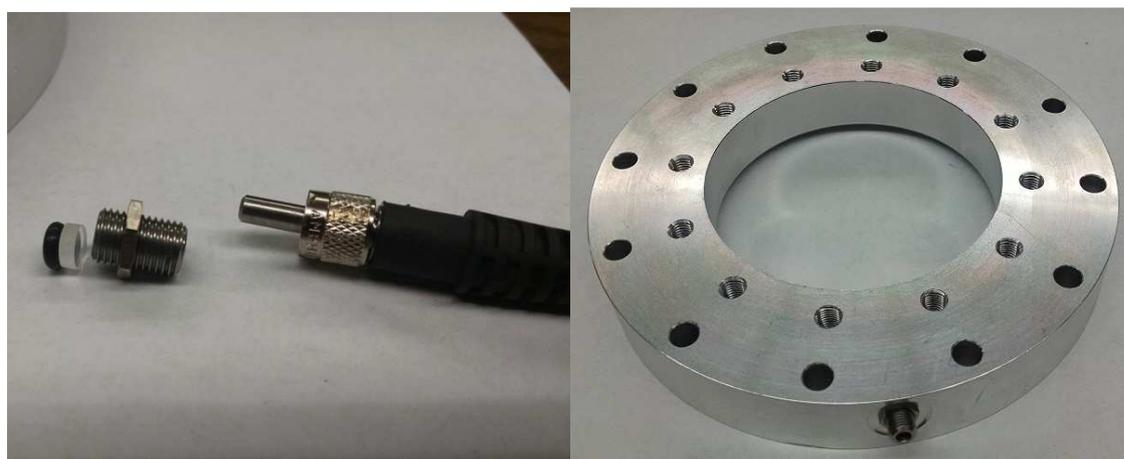
**Figure 3.31.** Fiber optic cable connecting PMT to pillbox window connects to a coupler that screws into the wall of the air side of the pillbox (left). The coupler compresses an o-ring between the pillbox and a quartz window, maintaining the integrity of the pressure seal when filling the waveguide with SF<sub>6</sub>. The coupler is shown screwed into the pillbox window in the right.
