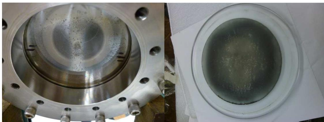
**Figure 3.28.** Metalization of a quartz window within the pillbox assembly. Sputtering is concentrated along the electric field component within the pillbox (left). Significant metalization (right) due to numerous sustained arcs degrades window transmission.
