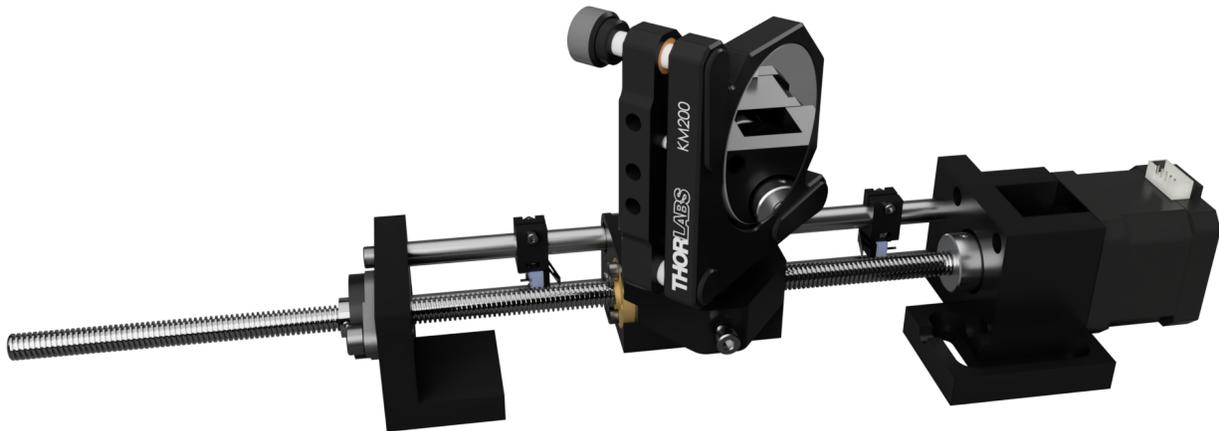
Figure 3.15: Linear stage for positioning a calibration mirror in front of the collection optics immediately after the plasma discharge. The stage was designed, 3D printed, and assembled by Ken Flanagan.
