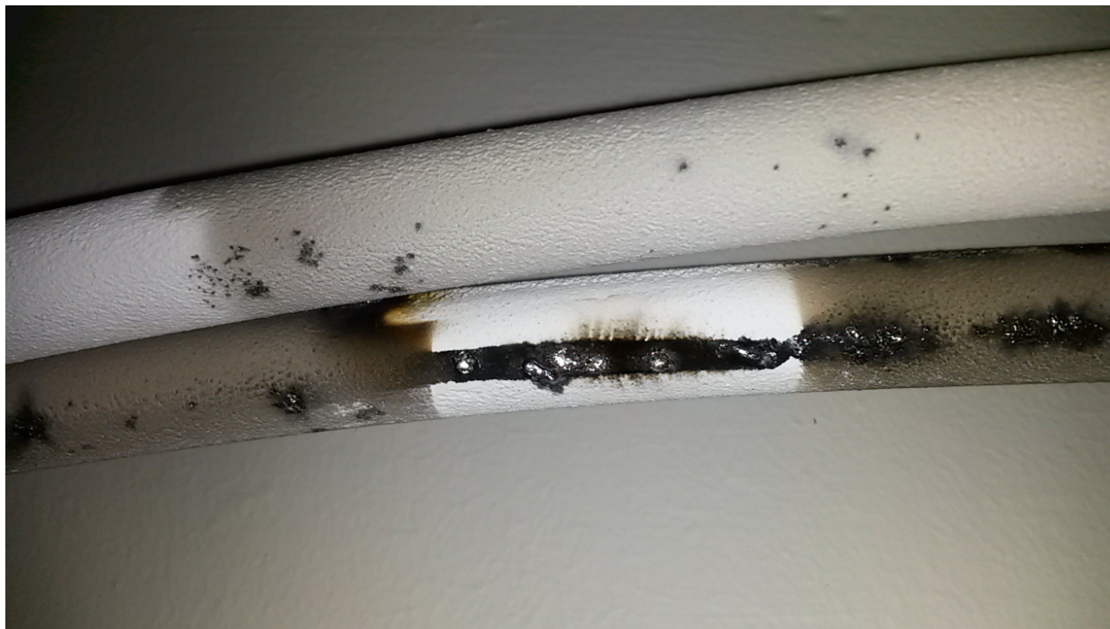
Figure 3.7: Scorch marks and arcing craters on the TREX 2015-2016 drive coils. The alumina coating was insufficient as an insulator. In addition to the visible damage, arcing to the coils also exerts a torque on the drive coil, which contributed to the eventual snapping of one of the TREX coil anchor wires.
