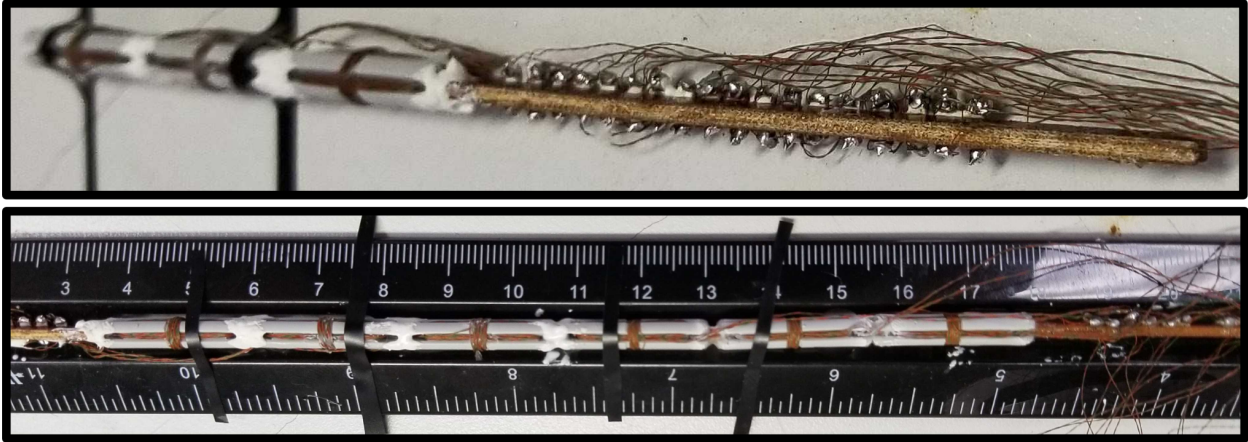
Figure A.9: Two examples that came out of the extended prototyping and testing of \dot{B} probes during TREX’s 2017 run. Both examples are made from carved LEGO pieces and hand-wound with magnetic wire. The prototype in the top picture shows early attempts at impedance-matching the probes, in this case by connecting the probe leads to resistors that have been glued to a scrap piece of phenolic. Lessons learned from these probe construction experiments went into the development of the standardized \dot{B} probes used in TREX 2018.
