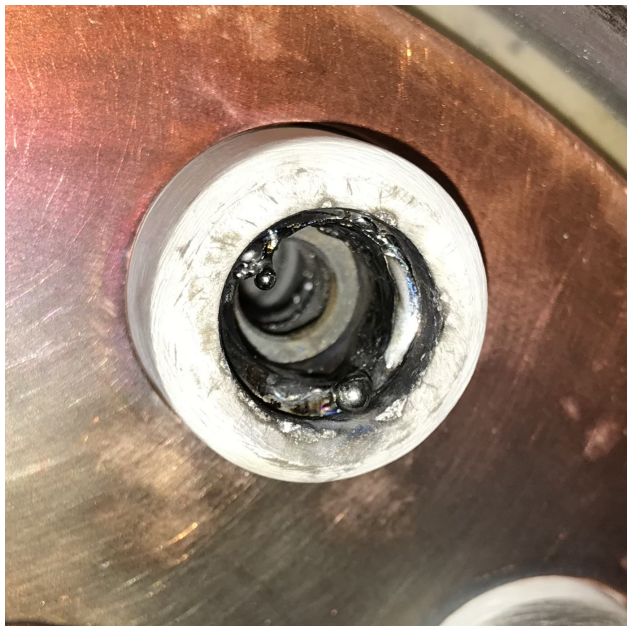
Figure D.5: Image of a washer gun in dire need of refurbishment. Visible also are the copper faceplate and white Boron-nitride shield. The gun anode clearly became molten and formed the two beads visible top-left and bottom. This image was taken after the flux rope experiment configuration, in which the gun anode was used also as a cathode to drive current across the vessel.
