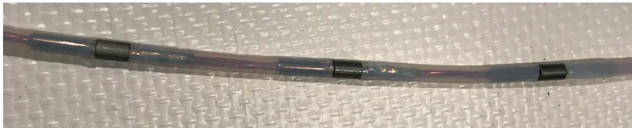
Figure C.2: One triple probe segment of four in a hanging array, centered at R = 10, 30, 50, and 70 cm. The plasma-facing molybdenum probe tips are jammed onto the stainless steel cylinder springs, which are soldered then to the copper wire. This type of press fit connection obviated the need for spot welding. Such a probe was never put to good use because of a failure in the CT switch stack that ended the experiment early.
