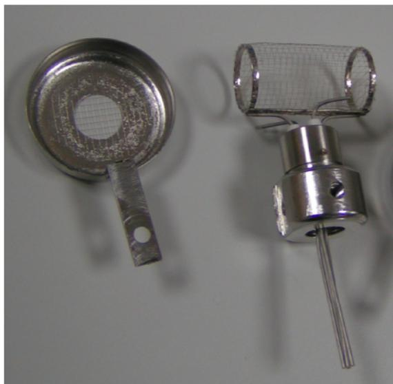
Figure 2.6: A photograph of the cylindrical mesh and endcap. Connections for the filament can also be seen, though no filament is attached.
