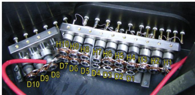
Figure 2.2: A photograph of the ANPA channeltron detectors. The top row is positioned to collect hydrogen ions while the bottom row is horizontally offset to collect deuterium of similar energies. Channel labels indicate progression from low to high energy.
