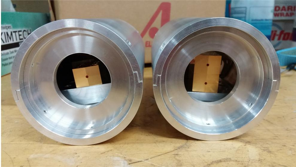
Figure 5.19 Photograph of planar diode mixer in mixer tube (left) and two mixer array for high wavenumber measurement experiments (right).
