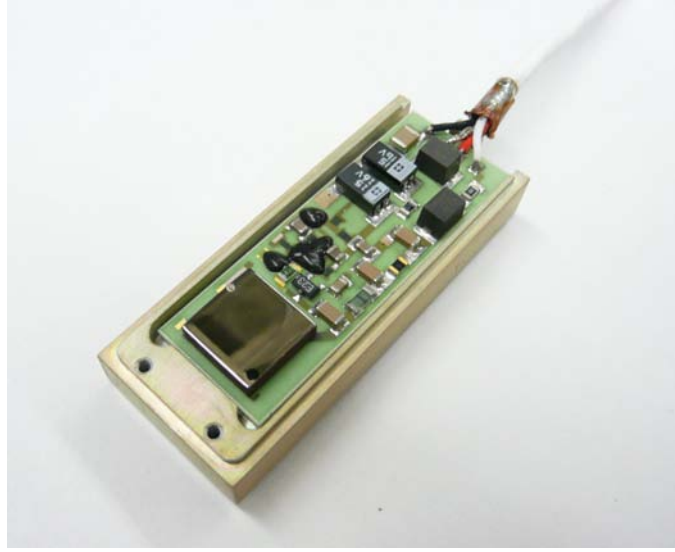
Figure 3.2: A CdZnTe hxr detector from eV Products with the cover removed.
