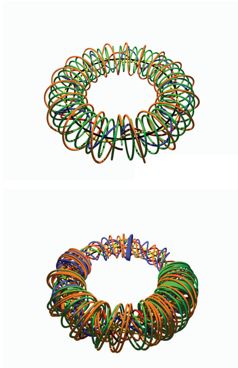
Figure 1.4: These two images show the effects of stochastic field line wandering. The first image is the ideal (fluctuation free field), a set of nested toroidal helices. The second plot shows the distortion caused by tearing modes and reconnection. Line coloration in the second image is based on the origin of the field line, and coincides with the coloration in the first image. Note change in radius, particularly for the orange, blue and green field lines.
