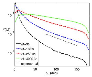
**Figure 1.** pdf of rotations in the magnetic field direction,  $P(\Delta\theta)$ , for the solar wind with measurement intervals of  $\Delta t \in \{1, 16, 256, 4096\} \cdot 3$  s (measured by the *WIND* spacecraft). While part of the tail ( $\Delta \theta > 60^{\circ}$ ) may be fit by an exponential function (straight line in the plot), the bulk of the pdf ( $\Delta \theta < 60^{\circ}$ ) varies drastically with  $\Delta t$ .
