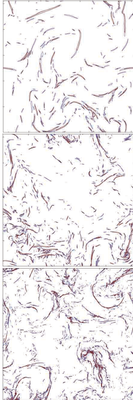
Fig. 3.— Contours of current density in an arbitrary plane perpendicular to the guide field. Contours are taken at j_{\text{thr}}/j_{\text{rms}} = 2 (blue) and j_{\text{thr}}/j_{\text{rms}} = 3 (red) for increasing Reynolds number (from top to bottom, Re = 1000, 3200, and 9000 ).
