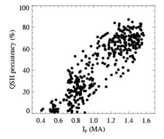
**Figure 3.** Persistency of the QSH phase as a function of plasma current. Persistency is defined as the fraction of the plasma current flat-top featuring a QSH phase. The highest current persistency exceeds 80%.
