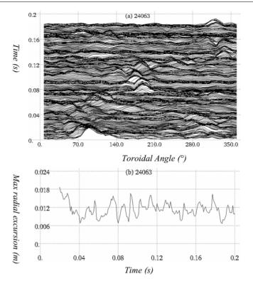
**Figure 1.** Radial displacement (a.u.) of the last closed magnetic surface due to m = 1 modes in shot 24063 as a function of the toroidal angle and of time (vertical direction). (b) Absolute maximum radial displacement (m) of the plasma as a function of time.
