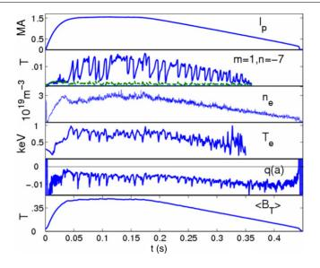
**Figure 2.** High current RFX-mod discharge #24063. From top: plasma current; amplitude of m = 1, n = -7 and (dashed line) average amplitude of 'secondary' modes m = 1 n = -8/-14;  $n_e$  (m<sup>-3</sup>);  $T_e$  from double SXR filter; q(a) and finally average toroidal flux.
