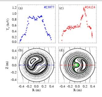
**Figure 4.** Electron temperature profiles from Thomson scattering diagnostic for (*a*) a high  $T_e$  plateau case and (*c*) a localized  $T_e$  structure, together with the corresponding Poincaré plots (*b*) for a SHAx case and (*d*) for the dominant m = 1, n = -7 magnetic mode preserving the island separatrix.
