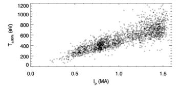
Figure 5. Electron temperature versus plasma current.
