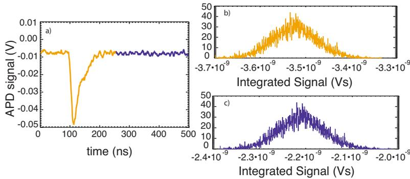
FIG. 3. (Color online) (a) A pulse of the LED as seen by an APD. The first half of the raw signal is integrated to get the light signal (orange). The second half of the light signal is integrated to get a baseline dark signal level (blue). Histograms of the 100 000 pulses for the (b) light and (c) dark signals are shown.
