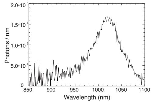
FIG. 2. Photons output by the pulsed LED and measured by the InGaAs absolutely calibrated detector at the monochromator exit. Measurements show a peak wavelength of 1020 nm with a full width at half maximum of 70 nm.
