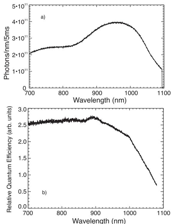
FIG. 6. (a) Number of photons collected as a function of wavelength in a 5 ms period for the absolute APD detector. (b) Relative QE of the APD.
