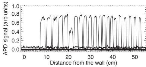
FIG. 1. The radial scan measures both the location and radial resolution of each polychromator view. The sixth channel shows the lower signal, which is due to a problematic detector at that location.
