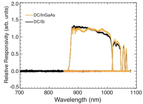
FIG. 5. (Color online) Instrument function, which is the product of transmission and QE, for a four channel polychromator.
