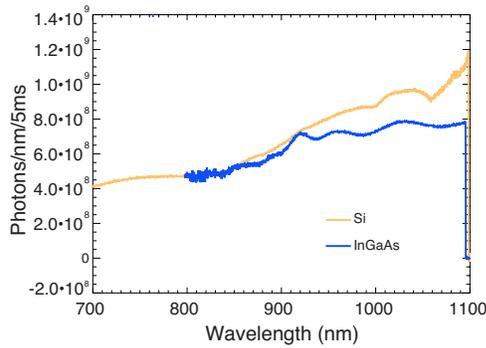
FIG. 4. (Color online) Number of photons collected as a function of wavelength in 5 ms period for Si and InGaAs detectors.
