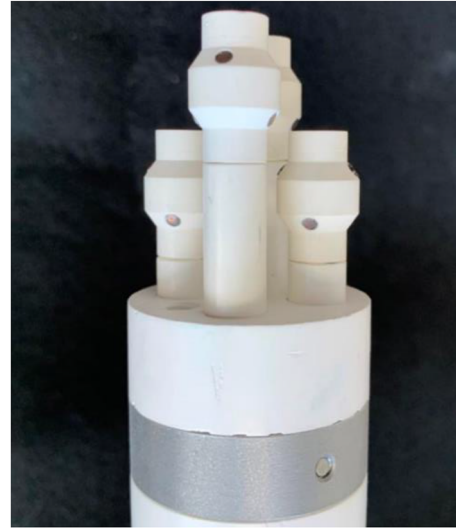
FIG. 1. Image of the completed tetrahedral Mach probe with four stalks, with molybdenum tips in place and the return electrode ring at the bottom.
