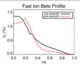
**Figure 9.** Fast ion  $\beta$  profiles from before (black solid) and after (red dashed) the sawtooth crash.
