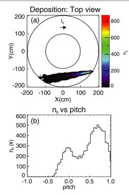
**Figure 6.** Initial deposition of beam injected fast ions in (*a*) space and (*b*) pitch (positive is co-current, negative is counter current). The initial pitch deposition peaks at  $\sim 0.68$ . Later in time the pitch is much more strongly peaked at  $\sim 0.8$ .
