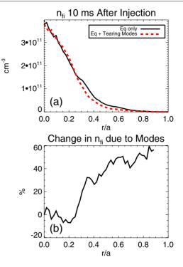
**Figure 7.** Fast ion density with and without tearing modes (*a*) and relative difference between the two profiles (*b*). Note that there were no test particles outside  $r/a \approx 0.9$  in the simulation.
