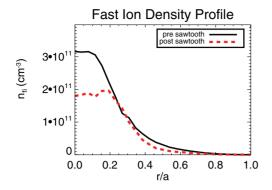
**Figure 8.** Fast ion density profile before (black solid) and after (red dashed) the sawtooth crash.
