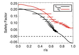
**Figure 4.** Magnetic safety factor (black) and effective safety factor of the fast ion guiding centre for a pitch = 1 (co-current), 25 keV hydrogen ion (red). The approximate island widths for the m = 1 modes are also shown.
