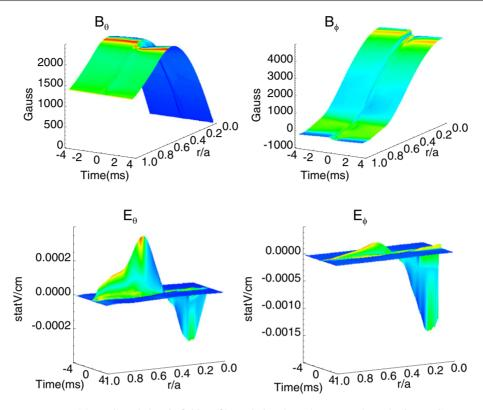
Figure 3. Magnetic and electric field profile evolution through a sawtooth crash (time = 0).
