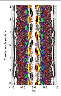
**Figure 5.** Toroidal puncture plot of the magnetic field (black) and five separate 25 keV hydrogen fast ion trajectories launched at various radii (coloured). The core-most ions (orange and yellow) are clearly well confined while those launched in the mid radius (red) are stochastic.
