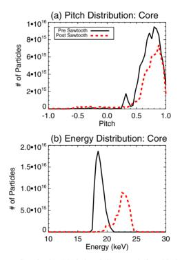
**Figure 10.** Core fast ion (*a*) pitch and (*b*) energy before (black solid) and after (red dashed) the sawtooth crash. The pitch increases due to acceleration from the mean  $E_{\parallel}$  and average energy increases by about 5 keV.
