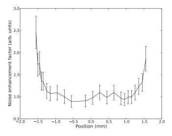
FIG. 3. Typical relative spatial profile of noise enhancement factor, measured by scanning a 0.1 mm diameter spot ( $\lambda = 1064$  nm) across the active area.
