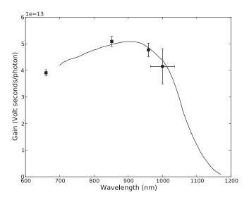
FIG. 5. Gain of an APD measured at the four LED wavelengths with characteristic curve fit.
