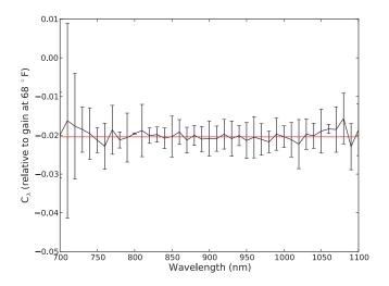
FIG. 2. Linear fit coefficients,  $C_{\lambda}$ , for the temperature dependence of APD gain. The mean value is indicated by the red line.
