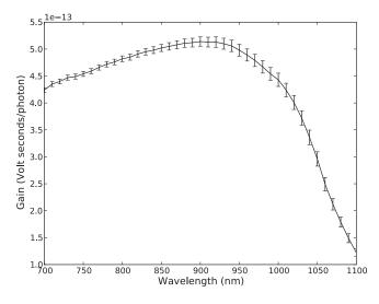
FIG. 1. Measured gain for one of the reference APDs. This is the dc gain value for a continuous light source.
