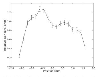
FIG. 4. Relative spatial profile of gain, measured by scanning a 0.1 mm diameter spot ( $\lambda = 1064$  nm) across the active area.
