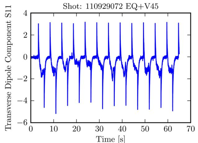
FIG. 8. A time series measurement of the  $S_{1,1}(r=a)$  mode of  $\mathbf{B}_{resp}$ . The spikes in the signal are due to the fast switching and are neglected in the pulse decay analysis.
