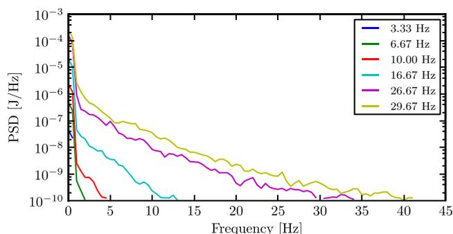
FIG. 12. Power spectral density calculated from the time series of the total response field magnetic energy (summed over spherical harmonic modes). The EQ + CD + V45 case is shown.
