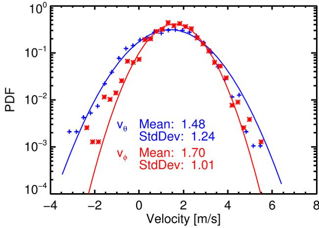
FIG. 3. Probability distribution function of LDV measurements of both  $v_\theta$  and  $v_\phi$  located at  $r=0.448$  m,  $\theta=0.60$  rad in the unconstrained flow (located just above the region between one of the impellers and the wall). The solid curves are Gaussian curve fits to the distributions.
