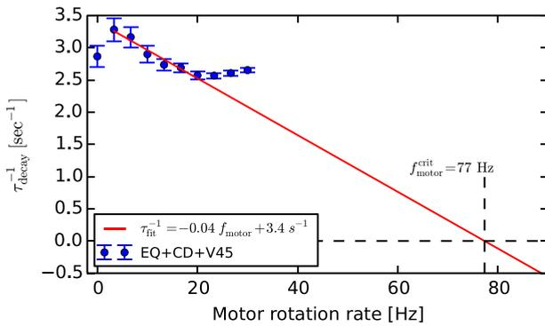
FIG. 14. A plot of the inverse pulse decay times as a function of motor rotation rate for the optimum flow configuration. The first six points, which show a clear linear descent, are used in a linear fit extrapolated to zero decay rate. The predicted threshold for self-excitation from this technique has a motor rotation rate of 77 Hz though subsequent measurements show that the decay time reaches a minimum long before this rotation rate.
