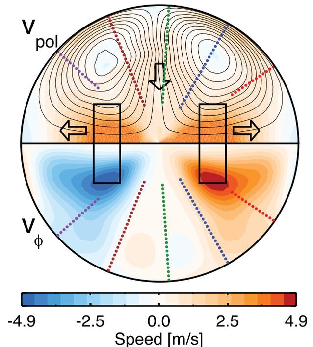
FIG. 2. A contour plot of the mean velocity field reconstructed from Laser Doppler Velocimetry (LDV) measurements in the water experiment with an unconstrained flow. Measurement locations are indicated by dots.
