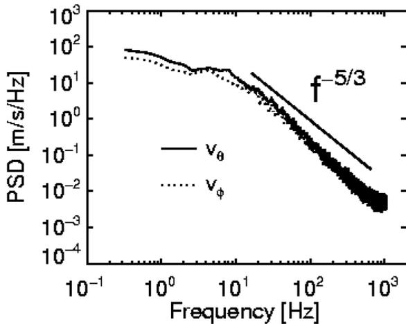
FIG. 4. The velocity power spectral density measurements of  $v_\theta$  and  $v_\phi$  at the same location described in Fig. 3 for the unconstrained configuration. The impeller rotation rate is 16.7 Hz. The measurements were taken over the course of 30 s and so the spectrum is poorly resolved at the lower frequencies. The spectrum is consistent with the  $f^{-5/3}$  power-law scaling predicted for Kolmogorov turbulence.
