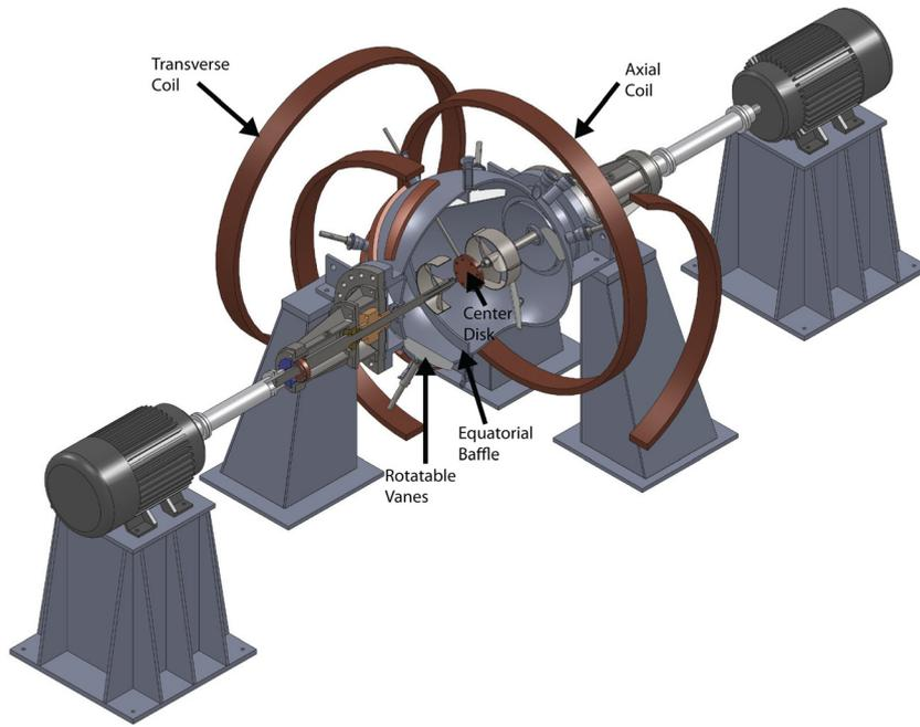
FIG. 1. Schematic of the liquid sodium vessel, impeller assemblies, motors, applied field coils, and boundary flow constraints.
