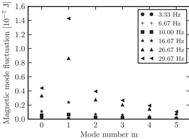
FIG. 13. Response field magnetic energy fluctuations (rms amplitude) calculated in terms of  $m$  spherical harmonic mode number (summed over  $\ell$ ). The EQ + CD + V45 case is shown.
