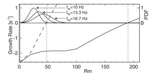
FIG. 6. Kinematic growth rate versus Rm for the mean flow measured in the water experiment (solid line) and an optimized flow (dashed line). The vertical lines identify  $Rm_{\rm crit}$  for each case. The PDFs of Rm for flows with three different impeller rotation rates are shown to demonstrate the increasing overlap of the ranges of Rm and  $Rm_{\rm crit}$ .
