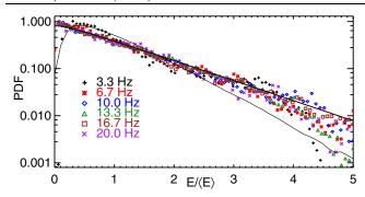
FIG. 7 (color online). The PDF of the energy in the transverse dipole field for several impeller rotation rates. The thick line is an example Poisson distribution. The thin line represents the energy distribution if the magnetic fluctuations were Gaussian.
