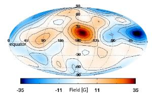
FIG. 3 (color online). Contours of  $B_r(\theta, \phi)$  measured on the surface of the sphere. The applied field is subtracted from the measurements. This snapshot of the measured field corresponds to an induced dipole field transverse to the drive shaft axis.
