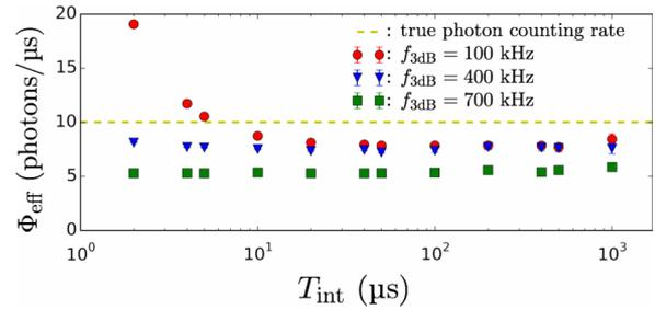
FIG. 3. Integration time vs effective photon counting rate for three different cutoff-frequencies. The true photon counting rate of  $10 \text{ photons}/\mu\text{s}$  corresponds to a typical expected signal level.
