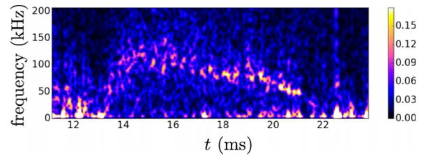
FIG. 6. Spectrogram for C III 229.7 nm electron impact emission observed in the edge of a 400 kA RFP plasma. The color represents the amplitudes with respect to the DC components.
