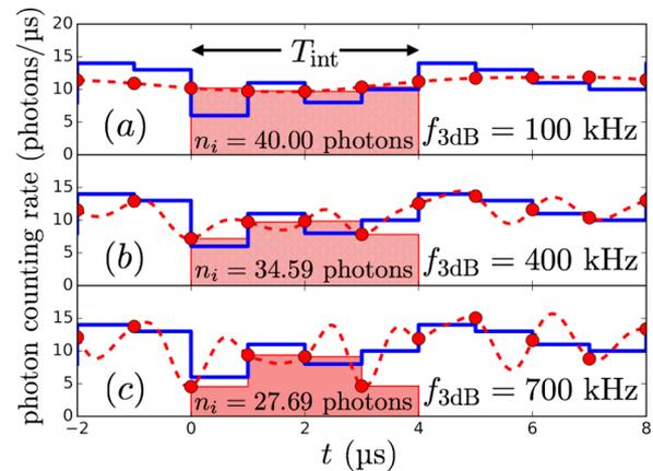
FIG. 4. Synthetic photon counts measurement for three different filter cutoff frequencies.  $\Psi = 10 \text{ photons}/\mu\text{s}$ ,  $T_{\text{int}} = 4 \mu\text{s}$  and  $N_i = 35$  photons. The blue lines represent the true photon counting rate. The red points represent digitized values. The red shaded areas represents  $n_i$  for each cutoff-frequency. The area under the blue line between  $0 \mu\text{s}$  and  $4 \mu\text{s}$  corresponds to  $N_i$ .
