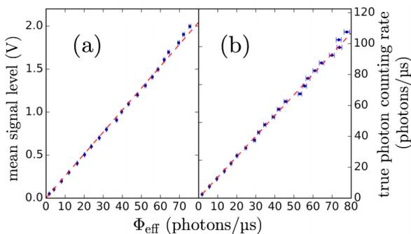
FIG. 2. (a) The effective photon counting rate measurement. An integrating sphere was used for a DC light source. (b) The simulation result for the relation between the photon counting rate and the effective photon counting rate. The simulation parameters,  $\mu$ , and  $l$  were chosen to match the specifications of the PMT<sup>8</sup> used in the measurements.  $f_{3\text{dB}} = 400 \text{ kHz}$  for both (a) and (b).
