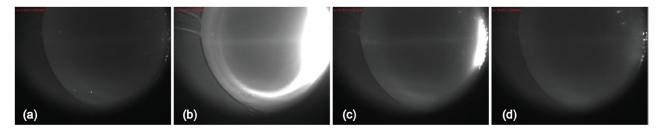
**Figure 12.** Time evolution of the PWI due to the application of a RMP. The data are from discharge 1140610079 characterized by  $I_p \simeq 500$  kA and RMP phase  $\simeq -2.7$  rad. In (a) the plasma is rotating, in (b) a RMP with  $B_r^{n=1}/B(a) \simeq 7\%$  is applied, in (c) the amplitude of the RMP is reduced to  $B_r^{m=1}/B(a) \simeq 3\%$  and in (d) there is no RMP but the plasma is still locked in the same position.
