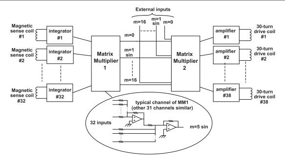
Figure 3. A schematic of the feedback-controlled error-field correction system for the poloidal gap on MST.
