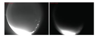
**Figure 13.** On the left visible and near infrared emission, on the right emission observed with a  $D_{\alpha}$  filter. Both the discharges have the same  $I_p$ ,  $n_e$  and both have an applied RMP of amplitude  $B_r^{m=1}/B(a) \simeq 9$ % and phase  $\simeq -1.2$  rad.
