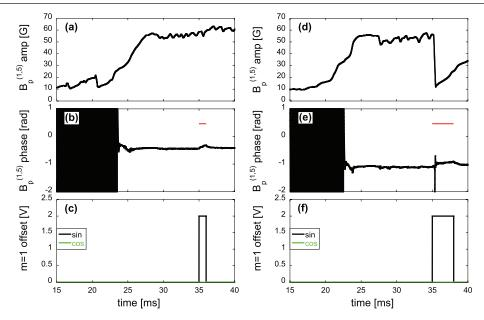
**Figure 8.** Examples of RMP applied when the plasma is already locked. The plots are the time evolution of: (a) and (d) amplitude of poloidal component of the core mode, (b) and (e) its phase and (c) and (f) the amplitude of the requested offset to the active feedback system. On the left a case with a RMP of  $B_r^{m=1} \simeq 120$  G applied for 1 ms (1130821026), on the right applied for 3 ms (1130821038). In (b) and (e) the red line corresponds to the requested locking phase.
