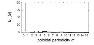
**Figure 4.** *m* radial mode spectrum during the application of a m = 1 RMP.
