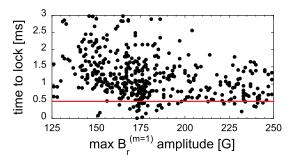
**Figure 11.** *Time to lock* as function of the amplitude of  $B_r^{m=1}$  measured by the sense coils at the poloidal gap.
