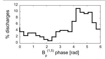
Figure 1. Probability to find the innermost resonant tearing mode locked at a particular poloidal phase angle at one toroidal location in MST during QSH state discharges. There is one locking event per discharge.
