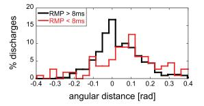
**Figure 9.** Histogram of the phase drift of the innermost resonant mode from 1 ms after the locking to the end of the plasma current flat top in case of RMP > 8 ms and of RMP < 8 ms.
