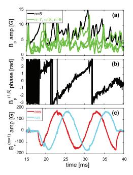
**Figure 16.** Application of a rotating RMP with a frequency of 100 Hz for a standard RFP discharge. (a) time evolution of the amplitude of the poloidal component of the core tearing modes, in black the m = 1, n = 6 mode, in green the m = 1,  $7 \le n \le 9$ ; (b) the phase of the poloidal component of the (1, 6) tearing mode; (c) the amplitude of the components of the m = 1 RMP applied.
