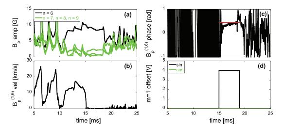
**Figure 14.** Example of a RMP applied during PPCD plasma showing (a) amplitude, (b) velocity and (c) phase of the poloidal m = 1, n = 6 magnetic mode. Plot (d) shows the requested m = 1 offset. PPCD is applied starting at 10 ms.
