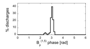
**Figure 6.** Distribution of the locking poloidal phase in a run day when a m = 1 RMP is applied with a phase of  $\pi$  rad.
