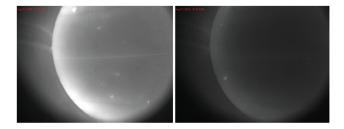
**Figure 15.** On the left visible and near infrared emission at the poloidal gap before the application of PPCD, on the right during the application of PPCD and a  $B_r^{m=1} \simeq 170$  G ( $B_r^{m=1}/B(a) \simeq 12$  %) RMP.
