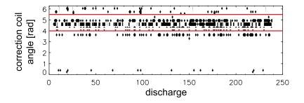
**Figure 17.** Saturation of the correction coils in discharges with  $I_p \simeq 500$  kA and  $B_t(a) = 0$  without applied RMP. The *y* axis is the angle of the correction coils, the *x* axis is discharge number and black points correspond to saturation of correction coils for that discharge in a time window between  $15 \le t \le 30$  ms. The two red lines highlight the most probable locking location area as suggested from the histogram in figure 1.
