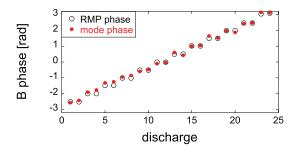
**Figure 7.** Locking poloidal phase for discharges with different RMP phase.
