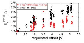
**Figure 10.** Amplitude of  $B_r^{m=1}$  measured by the sense coils at the poloidal gap as function of the offset requested to the active feedback. Points labeled in red deviate from linear dependence on the applied voltage due to the demand current exceeding a hardware limit in the feedback coil control.
