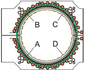
Figure 2. Cross-section of MSTs poloidal gap, the vertical insulated cut of the shell. The inboard side of the torus is to the left. Shown in cross-section is: heavy copper primary turns in red (A); 30-turn field error correction saddle coils in green (B); the vacuum vessel (C); and in-vacuum radial field sense coils (D).
