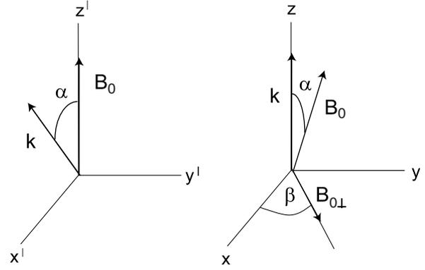
**Figure 1.** The Stix reference frame  $x'y'z'$  with  $z' \parallel B_0$  and  $k$  in the  $x', z'$  plane and the laboratory reference frame  $x, y, z$  with  $z \parallel k$  and  $x$ - and  $y$ -axes fixed with respect to the experimental device. The spatially varying azimuth  $0 \leq \beta \leq 2\pi$  is the angle in the  $x, y$  plane between  $x$  and the direction of  $B_{0\perp}$ ,  $\alpha$  is the angle between  $k$  and  $B_0$ .
