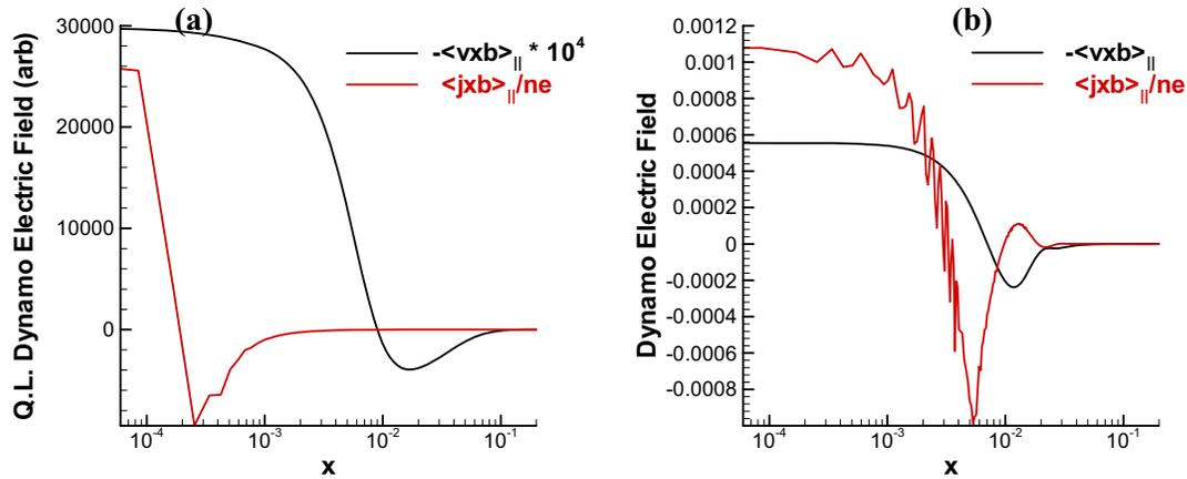
Fig.3. MHD and Hall dynamos vs. distance  $x$  from the resonant surface normalized to the equilibrium scale  $L$  during linear (a) and nonlinear (b) stages of tearing instability. Quasilinear computations (a) show strong and localized Hall dynamo, consistent with the analytical prediction. In nonlinear saturation (b), the Hall dynamo expands to the ion sound gyroradius scale  $\rho_s$ , and the two dynamos become comparable in magnitude.
