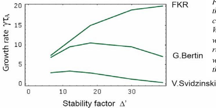
Fig. 7. Numerical calculations of the growth rate for different current profiles ( $\beta=0$ ,  $S=10^4$ ). Weakly reversed configurations with large  $\Delta'$  have smaller growth rates than deeply reversed states with small  $\Delta'$  that contradicts to the FKR analytic expression.
