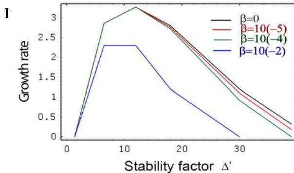
Fig. 8. Numerical calculations of the growth rate for different current profiles and values of  $\beta$  ( $S=10^4$ ). The  $m=0$  tearing instability driven by large  $\Delta' > 30$  are suppressed by finite  $\beta > 1\%$ .
