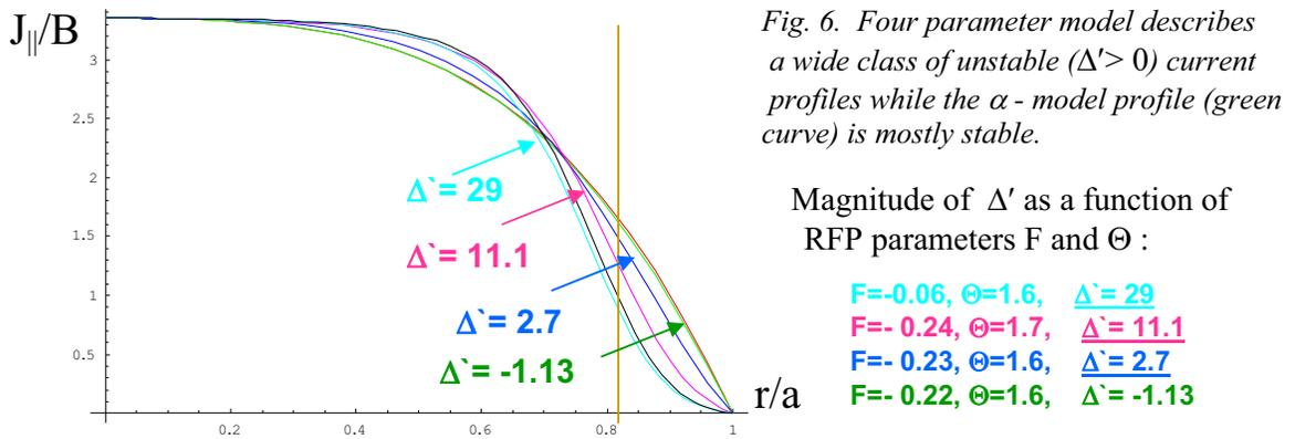
Fig. 6. Four parameter model describes a wide class of unstable ( $\Delta' > 0$ ) current profiles while the  $\alpha$ -model profile (green curve) is mostly stable.
