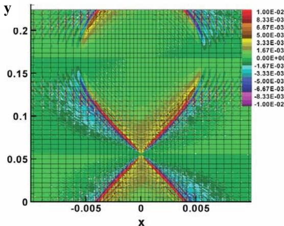
Fig. 5. Contours of local fluctuation-induced MHD dynamo.
