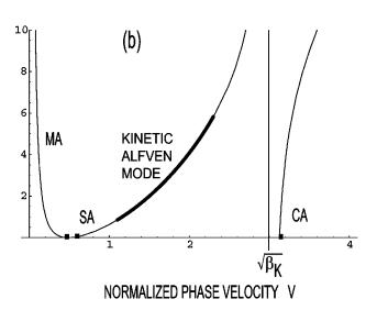
FIG. 1. Dependence of the lhs of the two-fluid dispersion relation (25) on the phase velocity V. Intersections with the horizontal line corresponding to the Hall term on the rhs of this equation yield three branches of oscillations [the magnetoacoustic (MA), shear (SA), and compressional (CA) Alfvén modes] modified on short scales by the two-fluid effects. (a) The case of  $\beta_k = \beta(1 + k^2 d_e^2) < \cos^2 \theta$ . (b) The case  $\beta_k > \cos^2 \theta$ .
