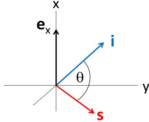
**Figure 2.** The incident and the scattered wave directions  $\mathbf{i} = \mathbf{k}_i/|\mathbf{k}_i|$  and  $\mathbf{s} = \mathbf{k}_s/|\mathbf{k}_s|$  ( $\theta$  is the scattering angle in the plane perpendicular to the vector  $\mathbf{e}_x = [\mathbf{s} \times \mathbf{i}]/\sin \theta$ ).
