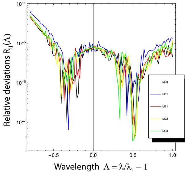
**Figure 6.** Plots of  $R_{ij}(\Lambda)$  vs  $\Lambda$  evaluated at 100 equidistant points within the interval  $-0.2 \leq \Lambda \leq 1$  at  $\theta = 140^\circ$ ,  $T_e = 25$  keV for five frequency-resolved Mueller matrix elements. The analytical and numerical results are in excellent agreement.
