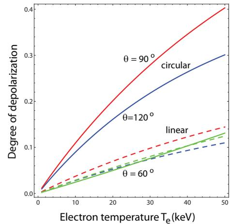
**Figure 4.** Depolarization degree vs  $T_e$  for three scattering angles:  $60^\circ$  (green),  $90^\circ$  (red) and  $120^\circ$  (blue) (solid lines: circular polarization at  $\chi = 45^\circ$ ; dashed lines: linear polarization at  $\psi = \chi = 0$ ).
