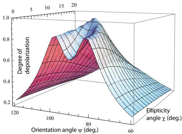
**Figure 3.** Depolarization degree vs orientation and ellipticity angles  $\psi$  and  $\chi$  at  $\theta = 90^\circ$ ,  $T_e = 10$  keV. There is a local maximum of  $D$  at  $\psi \simeq 82^\circ$  and  $\chi = 0$  (linear polarization), but the absolute maximum is reached at  $\psi = 90^\circ$  and  $\chi \simeq 9^\circ$  (elliptical polarization).
