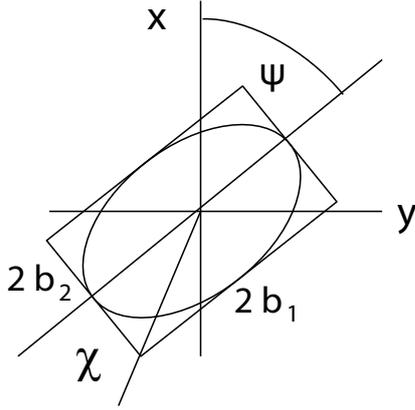
**Figure 1.** The azimuth of the polarization ellipse  $\psi$  (orientation angle) and the ellipticity angle  $\chi$  for purely monochromatic, fully polarized incident wave.
