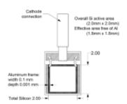
FIG. 1. Top-down view of photodiode showing 1  $\mu$ m thick aluminum frame (dark hatching) covering outer-most 100  $\mu$ m of the diode's 2.0 × 2.0 mm silicon active area. The silicon is mounted on a printed circuit board with a conducting anode base (hidden).
