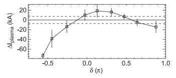
FIG. 4. Phase dependence of the change in cycle-averaged plasma current at the end of OFCD, relative to the change for OFCD off. Error bars refer to pulse-to-pulse variation in the measured current change. The two horizontal dashed lines show the pulse-to-pulse variation in measured current change for the same time period with OFCD off.
