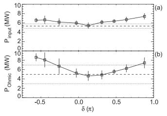
FIG. 7. Phase dependences of cycle-averaged, total (a) input power, i.e., the Poynting flux, and (b) the Ohmic input power, i.e., the input power minus the rate of change of magnetic energy from a relaxed state model, during the OFCD pulse. Error bars indicate pulse-to-pulse variability. Dashed horizontal lines are the same respective averages for OFCD off, and dotted lines indicate pulse-to-pulse variability for OFCD off.
