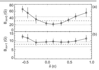
FIG. 6. Phase dependences of cycle-averaged (a) m = 0 ( $1 \le n \le 4$ ) mode amplitude and (b) m = 1 ( $6 \le n \le 15$ ) mode amplitude during the OFCD pulse. Error bars indicate pulse-to-pulse variability. Dashed horizontal lines are the same respective averages for OFCD off, and dotted lines indicate pulse-to-pulse variability for OFCD off.
