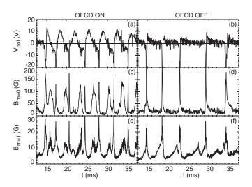
FIG. 5. Time dependences of the poloidal loop voltages for  $\delta \approx 5\pi/8$  OFCD (a) on and (b) off, m = 0 (toroidal modes  $1 \le n \le 4$ ) tearing mode amplitudes for (c) on and (d) off, and m = 1 ( $6 \le n \le 15$ ) amplitudes for (e) on and (f) off.
