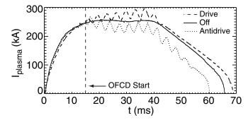
FIG. 1. Time dependences of the plasma current for three different pulses. The dashed curve is for the OFCD drive case, the dotted curve is for the OFCD antidrive case, and the solid curve is for the case with OFCD turned off.
