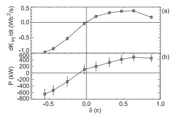
FIG. 3. Phase dependences of the cycle-averaged OFCD (a) helicity injection rate  $\langle 2\nu_t\phi_t\rangle$  and (b) input power  $\langle i_t\nu_t+i_p\nu_p\rangle$  (derived from the measured ac quantities). Error bars indicate pulse-to-pulse variability.
