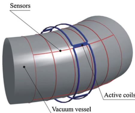
**Figure 57.** A section of the RFX-mod mechanical and magnetic front end, highlighting active saddle coils (blue) and magnetic sensors (red). In each toroidal location there are 4 active coils and 4 radial field sensors, for a total of 48 toroidal locations. Reproduced courtesy of IAEA. Figure from [646]. Copyright 2011 IAEA.
