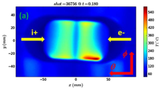
**Figure 68.** Graphite temperature by an IR camera in RFX-mod; the  $x$  axis corresponds to the poloidal direction, the  $y$  axis to the toroidal one. Reprinted from [579], Copyright 2017, with permission from Elsevier. CC BY-NC-ND 4.0.
