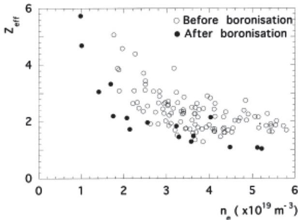
**Figure 70.** Effect of boronization on  $Z_{\text{eff}}$  in the RFX device. Reprinted from [573], Copyright 1999, with permission from Elsevier.
