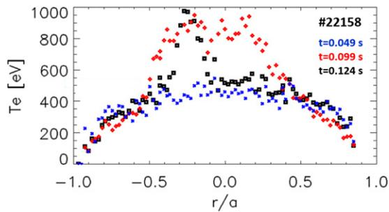
**Figure 23.** Comparison of the electron temperature profile in RFX-mod QSH (black squares QSH-DAX, red diamonds QSH-SHAX states) and MH (blue squares) plasmas.
