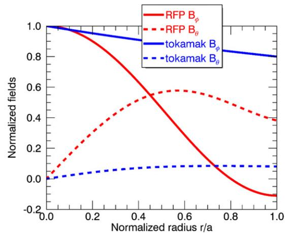
**Figure 2.** The toroidal ( $B_\phi$ ) and poloidal ( $B_\theta$ ) magnetic field profiles in RFP and tokamak.
