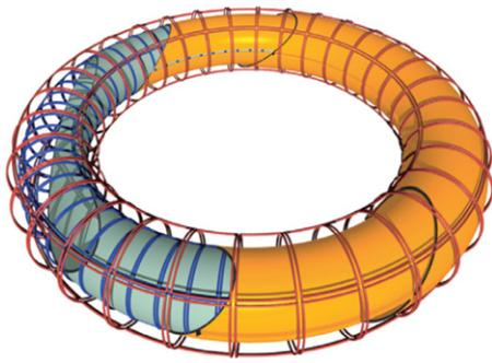
**Figure 56.** EXTRAP-T2R illustration showing the vacuum vessel (grey), the copper resistive wall (orange), the radial magnetic field sensors placed between the vessel and resistive wall (blue) and the active coils outside the resistive wall (red). Reproduced courtesy of IAEA. Figure from [545]. Copyright 2013 IAEA.
