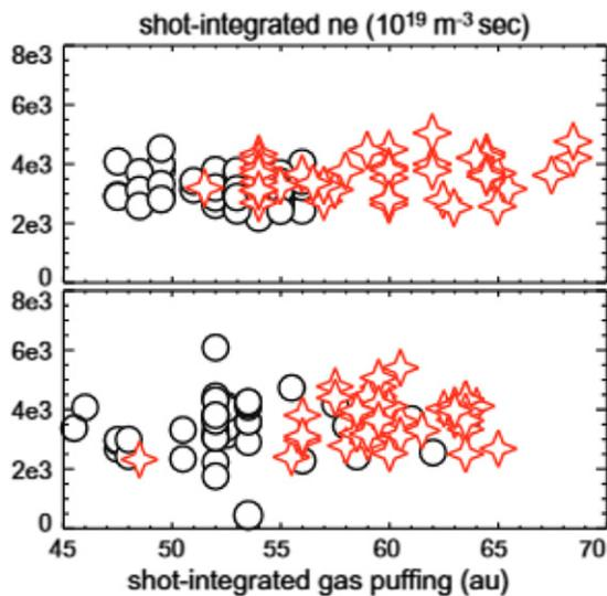
**Figure 69.** Electron density integrated during the current flat-top as a function of the total number of particles puffed in the MST device before (black circles) and after (red stars) boronization. Reprinted from [587], Copyright 2013, with permission from Elsevier.
