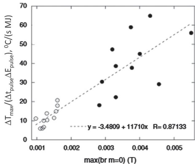
**Figure 67.** Evolution of maximum wall temperature in RFX-mod as a function of  $m = 0$  maximum radial field. Empty circles: with feedback; black circles: without feedback. Reprinted from [79], Copyright 2007, with permission from Elsevier.
