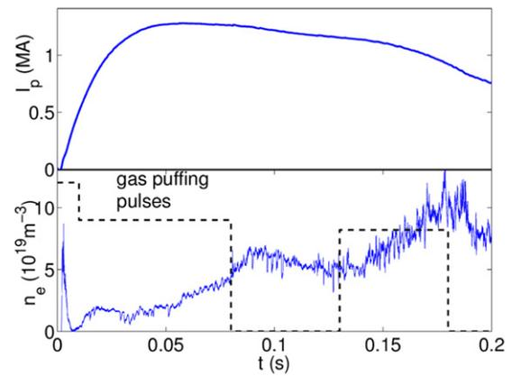
**Figure 71.** Time evolution of plasma current (top) and electron density (bottom) after lithization in RFX-mod. Pulses of puffed gas are superimposed (dashed), showing the good response of density. Reproduced courtesy of IAEA. Figure from [575]. Copyright 2013 IAEA.
