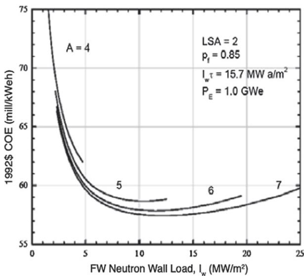
**Figure 80.** 1 GWe RFP power-plant COE as a function of FW neutron wall load,  $I_w$ , for several plasma aspect ratios,  $A = R/a$ . The plant availability is assumed to be  $p_f = 0.85$ . [643] 2009, reprinted by permission of the publisher (Taylor & Francis Ltd, <http://www.tandfonline.com>.)
