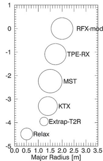
**Figure 1.** Cross sections of the RFP devices listed in table 1.
