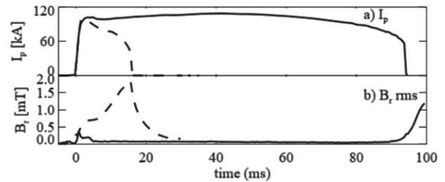
**Figure 58.** EXTRAP-T2R pulse showing the discharge current and total radial field amplitude at the sensor coil array for a discharge without control (dashed line) and with active control (line).
