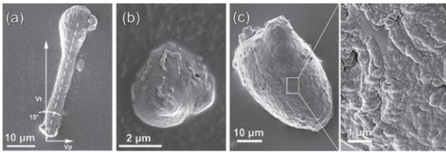
**Figure 72.** Examples of SEM analysis of dust particles collected post-mortem in EXTRAP-T2R by adhesive tape. Particles are mainly spheroids covered by deposits (b) with granular morphology (b) and (c). Few elongated particles also observed (a). Reproduced from [603]. © IOP Publishing Ltd. All rights reserved.
