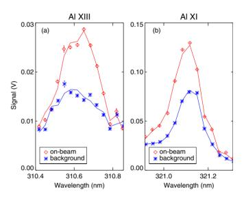
**Figure 1.** On-beam (charge-exchange + electron-impact) and background (electron-impact) data along with best-fit model results (solid lines) for (*a*) Al XII *n* = 11–10 transition at  $\lambda \sim 310.65$  nm (sh#1110301068) (*b*) Al XI *n* = 10–9 transition at  $\lambda \sim 321.05$  nm (sh#1110509028). From calibration,  $1V \sim 9 \times 10^8$  photons s<sup>-1</sup>. The ion temperatures obtained from the model are  $T_{AI^{+13}} \sim 1.3$  keV and  $T_{AI^{+11}} \sim 1.1$  keV.
