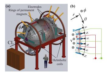
FIG. 1. The MPDX: (a) a sketch of the experiment; (b) the electrode configuration near the wall for driving plasma velocity  $v_{\phi}(\theta)$ . The spherical system of coordinates  $(r, \theta, \phi)$  is shown. Center line (CL) corresponds to the axis of symmetry. Reprinted with permission from Phys. Plasmas **19**, 104501 (2012). Copyright 2012 American Institute of Physics.
