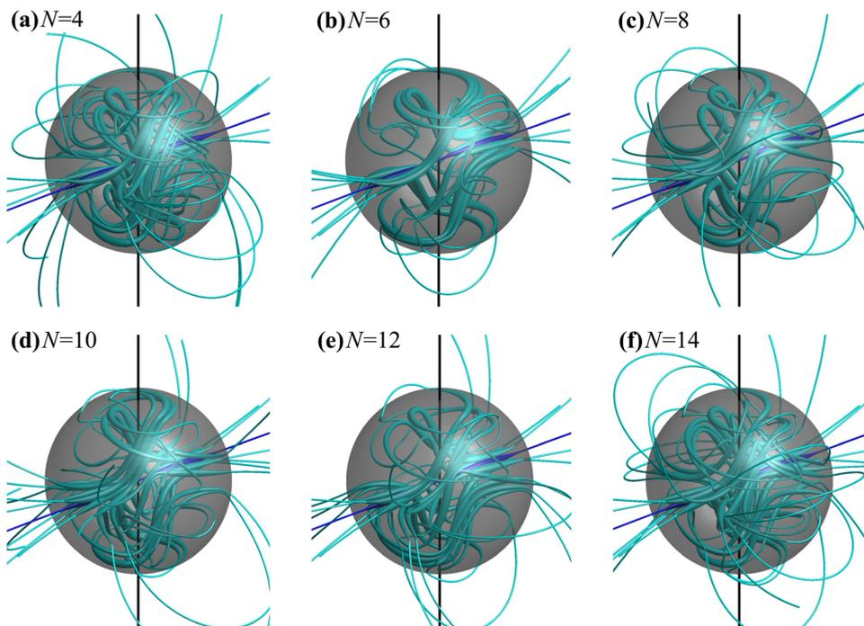
FIG. 13. Magnetic field lines of the fastest kinematic dynamo eigen-modes obtained at  $Rm=400$  for the optimized flows shown in Fig. 11. Thickness of the lines is proportional to the magnitude of the field. Vertical lines represent the axis of symmetry of the flows. Horizontal lines (shown in darker color) denote the axis of these equatorial dipole-like dynamo fields.
