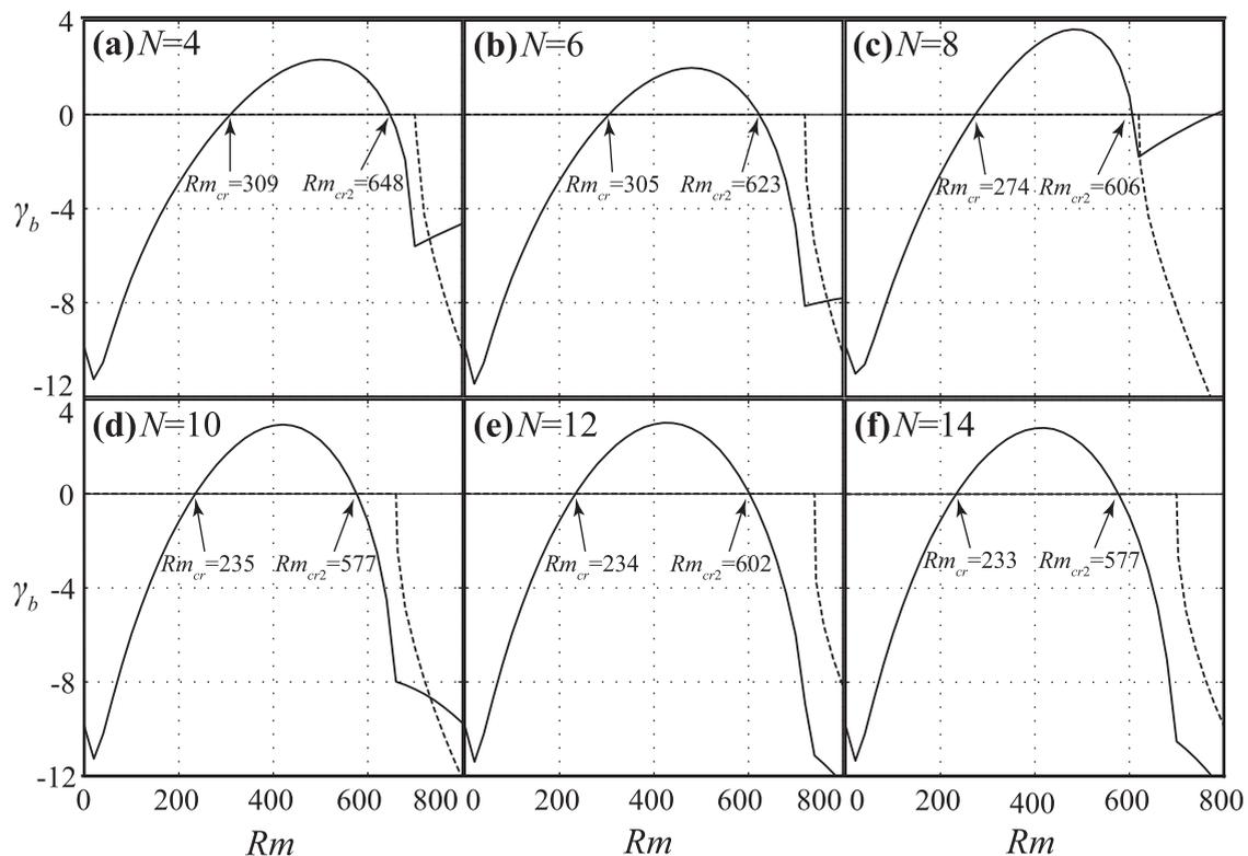
FIG. 12. Dependences of real (solid curves) and imaginary (dashed curves) parts of dynamo growth rate  $\gamma_b$  on magnetic Reynolds number  $Rm$  for the optimized flows shown in Fig. 11. Calculations are done for the fastest dynamo mode (with azimuthal mode number  $m = 1$ ).
