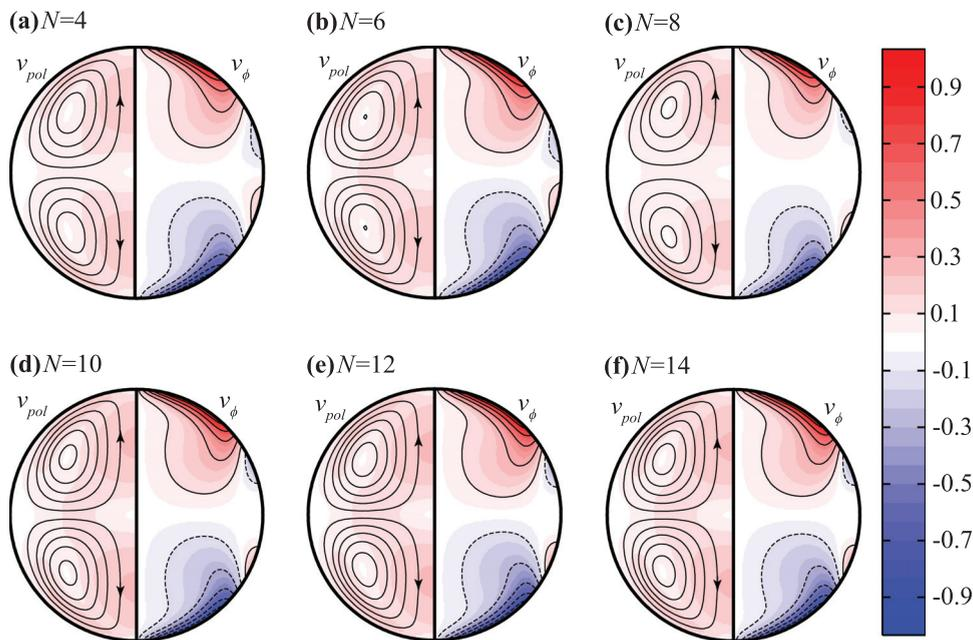
FIG. 11. Axisymmetric equilibrium flows corresponding to optimized driving velocities from Fig. 10 at fluid Reynolds number  $Re = 150$ . Notations are the same as in Fig. 3.
