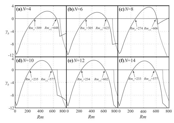
FIG. 12. Dependences of real (solid curves) and imaginary (dashed curves) parts of dynamo growth rate  $\gamma_b$  on magnetic Reynolds number Rm for the optimized flows shown in Fig. 11. Calculations are done for the fastest dynamo mode (with azimuthal mode number m = 1).
