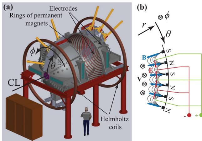
FIG. 1. The MPDX: (a) a sketch of the experiment; (b) the electrode configuration near the wall for driving plasma velocity  $v_\phi(\theta)$ . The spherical system of coordinates  $(r, \theta, \phi)$  is shown. Center line (CL) corresponds to the axis of symmetry. Reprinted with permission from Phys. Plasmas **19**, 104501 (2012). Copyright 2012 American Institute of Physics.
