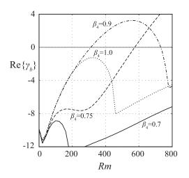
FIG. 7. Real part of dynamo growth rate Re{ $\gamma_b$ } as a function of magnetic Reynolds number *Rm* for fluid Reynolds number *Re* = 150 and different values of driving parameters  $\beta_4 = 0.7$  (solid curve),  $\beta_4 = 0.75$  (dashed curve),  $\beta_4 = 0.9$  (dashed-dotted curve) and  $\beta_4 = 1.0$  (dotted curve).
