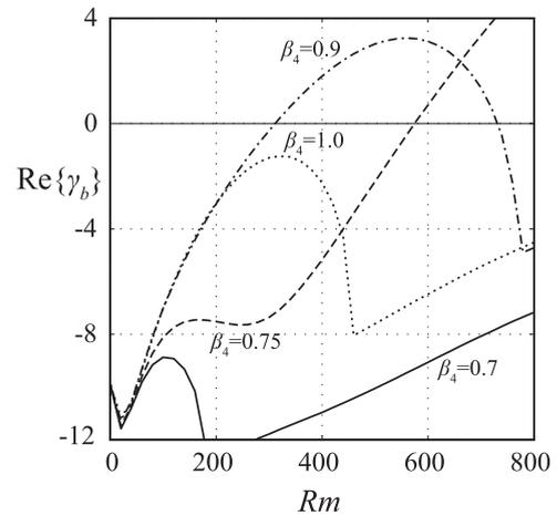
FIG. 7. Real part of dynamo growth rate  $\text{Re}\{\gamma_b\}$  as a function of magnetic Reynolds number  $Rm$  for fluid Reynolds number  $Re = 150$  and different values of driving parameters  $\beta_4 = 0.7$  (solid curve),  $\beta_4 = 0.75$  (dashed curve),  $\beta_4 = 0.9$  (dashed-dotted curve) and  $\beta_4 = 1.0$  (dotted curve).
