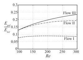
FIG. 5. Ratio of poloidal to toroidal kinetic energies  $E_{pol}/E_{tor}$  as a function of fluid Reynolds number *Re* for flows I, II, and III.
