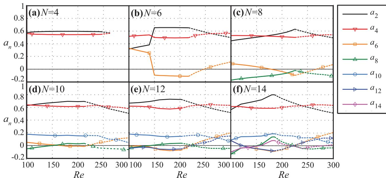
FIG. 9. Dependences of driving Fourier coefficients  $a_n$  on fluid Reynolds  $Re$  in optimized flows with different number of driving harmonics. Values of  $Re$  are scanned with step  $\Delta Re = 10$ . As in Fig. 8, solid curves correspond to the stable flows, dashed curves correspond to the marginally stable flows.
