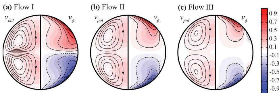
FIG. 3. Equilibrium structures of flows I, II, and III for fluid Reynolds number  $Re = 150$ . The left half of each figure shows stream lines of poloidal velocity  $v_{pol}$  superimposed on its absolute values depicted in colors, the right half shows a contour plot of azimuthal velocity  $v_\phi$  (dashed curves denote values of  $v_\phi < 0$ ). The vertical central lines represent the axis of symmetry.
