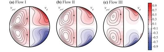
FIG. 3. Equilibrium structures of flows I, II, and III for fluid Reynolds number Re = 150. The left half of each figure shows stream lines of poloidal velocity  $v_{pol}$  superimposed on its absolute values depicted in colors, the right half shows a contour plot of azimuthal velocity  $v_{\phi}$ (dashed curves denote values of  $v_{\phi} < 0$ ). The vertical central lines represent the axis of symmetry.
