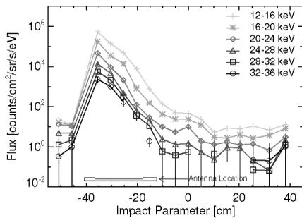
**Figure 2.** Radial profile of HXR flux looking at the face of the antenna with 85 kW of input power.
