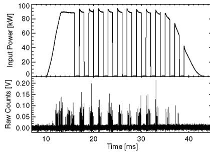
**Figure 3.** The rf power modulated at 500 Hz and the HXR response.
