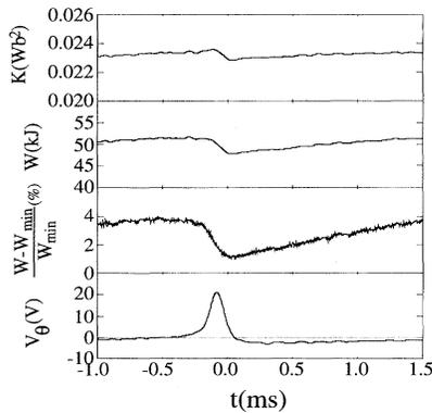
FIG. 2 The magnetic helicity  $K$ , magnetic energy  $W$ , and “excess energy”  $(W - W_{\min})/W_{\min}$  during one sawtooth cycle.  $W_{\min}$  is energy predicted by the BFM with a given  $K$  and  $\Phi_\phi(a)$ . Also shown is  $V_\theta(a)$  as a time reference.
