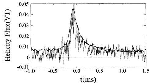
FIG. 4. Comparison between the measured fluctuation-induced helicity flux (dotted line) and the prediction (solid line) from local helicity balance at  $r = a - 5$  cm.
