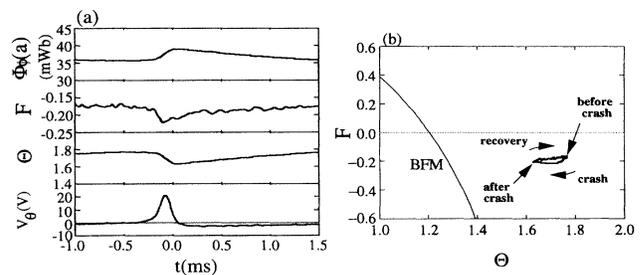
FIG. 1. (a) Ensemble-averaged toroidal flux  $\Phi_\phi(a)$ , pinch parameter  $\Theta$ , reversal parameter  $F$ , and voltage across the toroidal gap in the shell  $V_\theta(a)$  during one sawtooth cycle. The ensemble consists of 150 sawtooth oscillations. (b) Plasma trajectory during one sawtooth cycle. The BFM (Bessel function model) curve is the locus of predicted minimum energy states.
