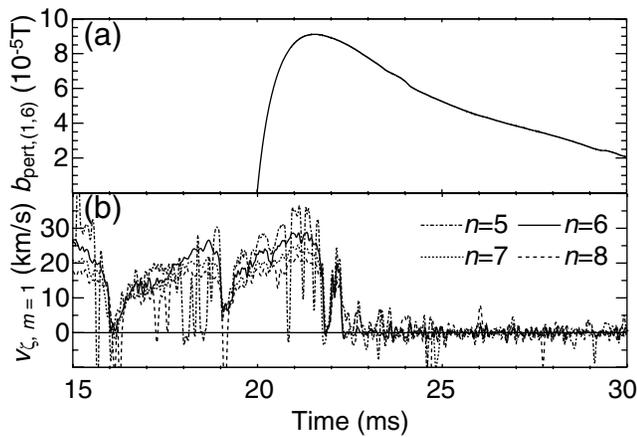
FIG. 6. Discharge with applied  $n = 6$  perturbation. (a) ( $m = 1$ ) component of ( $n = 6$ ) perturbation. (b) ( $m = 1, n = 5-8$ ) mode toroidal phase velocities
