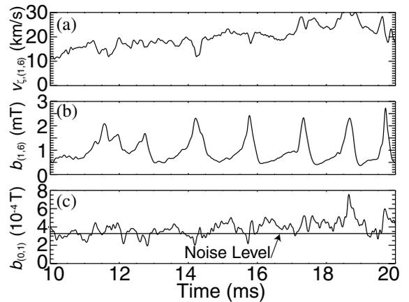
FIG. 5. Discharge with no ( $m = 0$ ) resonance. (a) (1,6) mode toroidal phase velocity. (b) (1,6) mode amplitude. (c) (0,1) mode amplitude.
