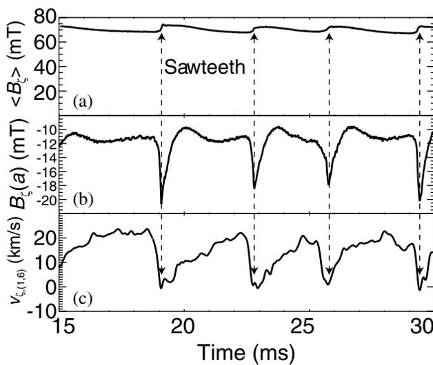
FIG. 1. (a) Volume averaged toroidal field. (b) Average toroidal field at plasma edge ( $r = a$ ). (c) Toroidal phase velocity of  $(1,6)$  mode, in a typical MST discharge.
