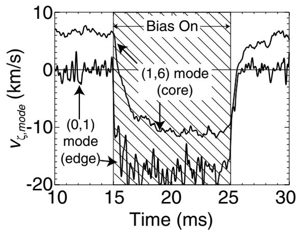
FIG. 2. Evolution of  $(1,6)$  and  $(0,1)$  mode toroidal phase velocities with edge biasing. The velocities are averaged over approximately 40 discharges.
