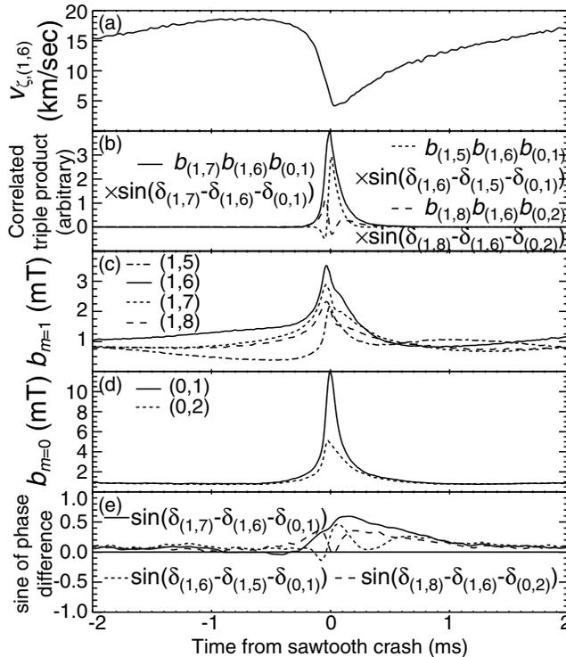
FIG. 4. Ensemble-averaged quantities for tripleproduct measurement. (a) (1,6) mode toroidal phase velocity. (b) Nonlinear triple products. (c) ( $m = 1$ ) mode amplitudes. (d) ( $m = 0$ ) mode amplitudes. (e) Phase factors.
