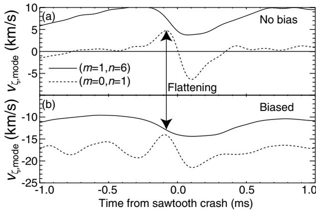
FIG. 3. Ensemble averaged toroidal phase velocities for the (1,6) and (0,1) modes in (a) normal and (b) biased cases. Note the difference in the vertical scales.
