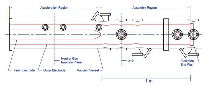
FIG. 2. (Color online) Drawing of the ZaP experimental apparatus is shown. The drawing identifies the key features — the acceleration region, assembly region, and the z = 0 plane. Zeeman splitting measurements are made through the bottom port at z = 0. A 1 m scale is included for reference.
