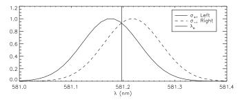
FIG. 1. The spectral intensity measured with a quarter wave plate and linear polarizer show the shift due to Zeeman splitting. The peak of the intensity shift between the right hand circularly polarized (dashed) and the left hand circularly polarized (solid) view is proportional to the magnetic field. The unshifted wavelength is shown for reference.
