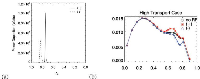
**FIGURE 1.** (a) Power Absorption versus radius calculated by GENRAY (b) corresponding  $E_{\parallel}$  spectrum. Notice the relative peak and the valley for the two different wave injection directions. Here, (+) indicates a positive  $n_{\parallel}$  spectrum and (-) indicates a negative  $n_{\parallel}$  spectrum.
