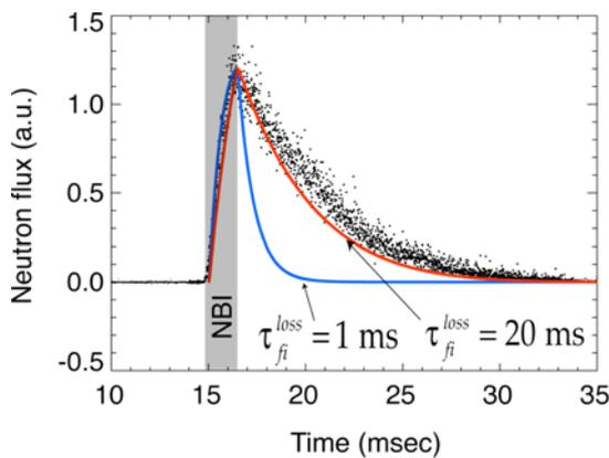
FIG. 1. Comparison of measured neutron signal (dots) and modeling (solid lines). The shaded area represents the NBI duration. The solid  $\tau_{fi}^{loss} = 20$  ms and  $\tau_{fi}^{loss} = 1$  ms lines show the fits for the corresponding fast ion confinement times.
