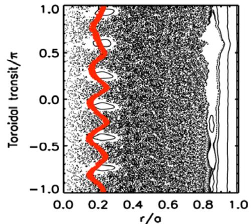
FIG. 2. Puncture plots of magnetic field line and ion guiding center (red) with the same starting point  $r/a = 0.20$ . The field line randomly wanders through the plasma volume while the fast ion stays attached to a flux surface.
