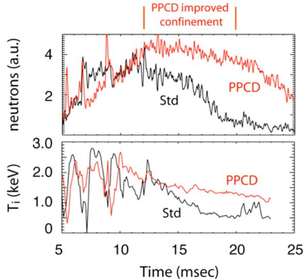
FIG. 5. Comparison of central ion ( $C^{+6}$ ) temperature and neutron flux in high  $I_p$  PPCD (red) and standard (black) plasma. PPCD is turned on at  $t = 10 \text{ ms}$  and a quiescent period lasts from  $t = 12 \text{ ms}$  to  $t = 20 \text{ ms}$ . The ion are anomalously heated prior to PPCD as result of magnetic reconnections (appear as discrete spikes on the signals).
