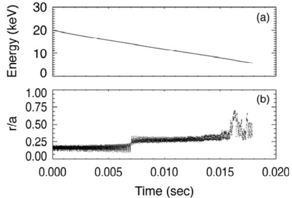
FIG. 3. Calculated time dependence of ion energy (a) and the position of the ion guiding center (b).
