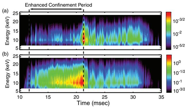
FIG. 4. (a) ANPA signal increases substantially after the end of an enhanced confinement period in which  $D_\alpha$  emission is reduced. Neutral density also increases dramatically at the end of this period, and after normalizing (b), the fast ion density is seen to be reduced after loss of confinement.
