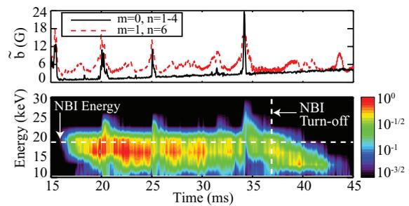
FIG. 6. Energization of the NBI hydrogen distribution is observed during sawtooth crashes, and decay of the distribution function can be measured after beam turn-off at 37 ms.
