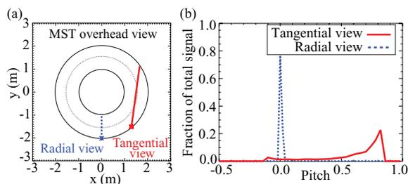
FIG. 2. The geometry of the ANPA viewports on MST (a) affects the pitch distribution sampled by the diagnostic (b).
