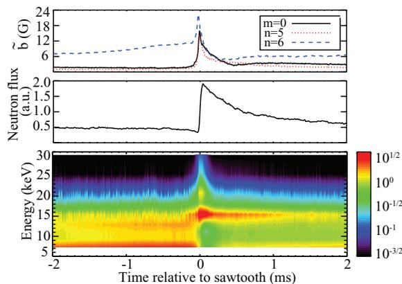
FIG. 5. After reduction of statistical noise by averaging 205 similar sawtooth events, energization of thermal deuterium ions during reconnection is observed on the ANPA. D–D neutron flux rises dramatically as signal moves into the higher ANPA  $D^+$  energy channels. These data were taken on the radial viewport and are calibrated for relative detector efficiency.
