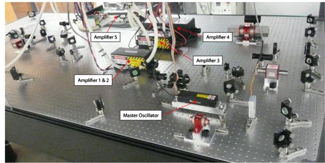
FIG. 4. (Color online) Optical table layout of high-repetition-rate pulse-burst laser system being commissioned for addition to the MST Thomson scattering system.
