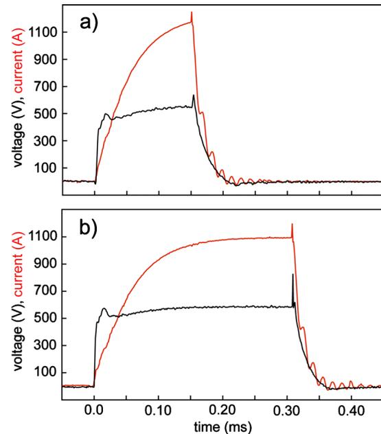
FIG. 2. (Color online) Voltage (black trace) and current (gray/red trace) applied to the largest flashlamp in the laser head to produce (a) one of fifteen 0.15 ms pulses and (b) one of five 0.31 ms pulses.
