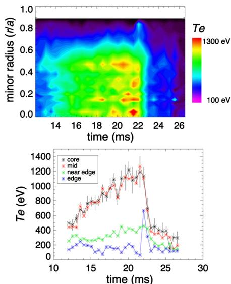
FIG. 3. (Color online) Thomson scattering measurement of electron temperature evolution during an improved confinement discharge. Both upper and lower plots are illustrations of the same data. Temperature in the core volume of the plasma steadily rises during the improved confinement period and then drops rapidly as the period ends.
