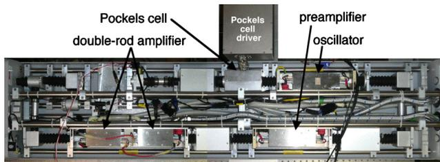
FIG. 1. (Color online) An overhead view of the Nd:YAG laser head.
