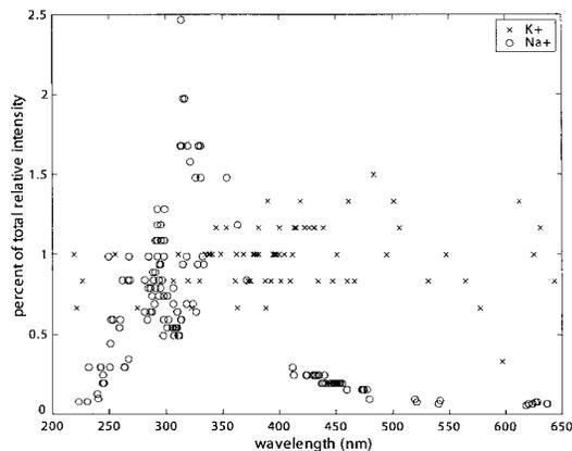
FIG. 3. Normalized  $\text{Na}^+$  and  $\text{K}^+$  emission intensities.
