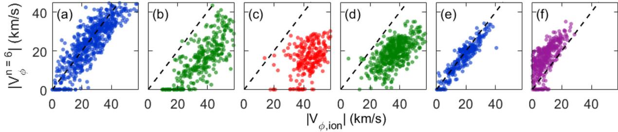
FIG. 6. Correlation between the  $m = 1, n = 6$  mode phase velocity and toroidal ion flow for all shots and times at (a)  $r = -16$  cm, (b)  $-6$  cm, (c)  $+4$  cm, (d)  $+8.9$  cm, (e)  $+17.8$  cm, and (f)  $+26.7$  cm. The dotted line represents a 1:1 correlation.
