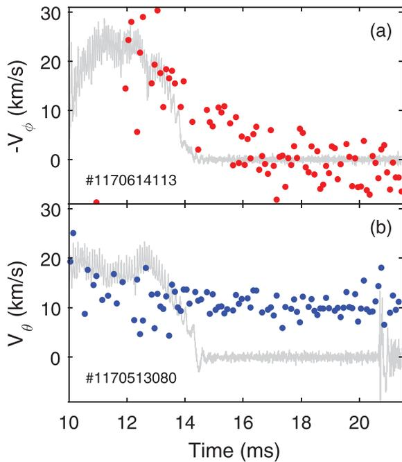
**FIG. 8.** Lines show the  $m = 1$ ,  $n = 6$  toroidal phase velocity for two similar shots [(a) and (b)]. Dots represent the measured ion flow near the resonant surface: (a) toroidal flow at  $r = -16$  cm and (b) poloidal ion flow at  $r = +17.8$  cm.
