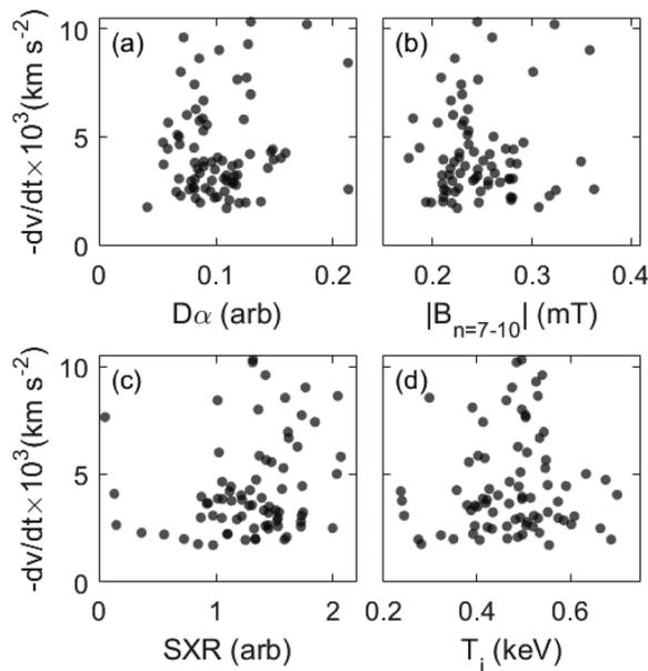
**FIG. 9.** Correlation between the  $(m, n) = (1, 6)$  mode deceleration and (a) neutral deuterium intensity, (b) combined rms mode amplitude for  $n = 7-10$ , (c) average soft X-ray emission during 18–20 ms, and (d) ion temperature.  $D_\alpha$  and SXR are uncalibrated. Each data point represents one shot.
