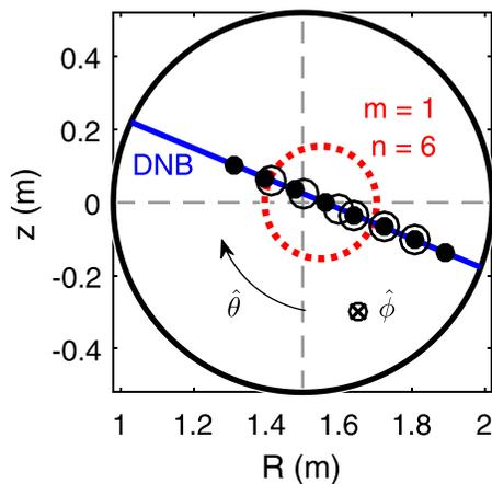
**FIG. 2.** A poloidal cross-sectional view of the MST with toroidal direction into the page and poloidal direction clockwise. Toroidal velocity measurement locations (open circles) and poloidal velocity measurement locations (solid circles) are shown along the path of the diagnostic neutral beam (blue line). The red dashed circle marks the location of the  $(m, n) = (1, 6)$  tearing mode resonant surface.
