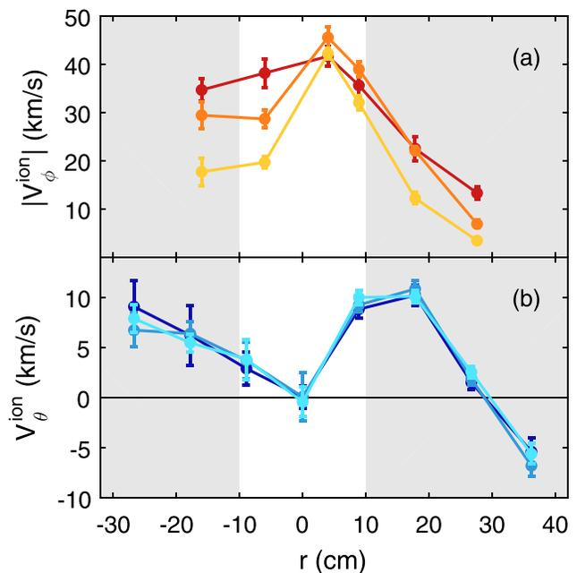
FIG. 4. (a) Toroidal and (b) poloidal flow profile evolution in time, averaged over several (4–9) shots for each location. Profile lines evolve from darkest to lightest tone, with time windows 12–14 ms, 15–17 ms, and 18–20 ms, respectively. Error bars represent the variation in the data from individual discharges. The shaded regions indicate the regions where tearing modes are resonant.
