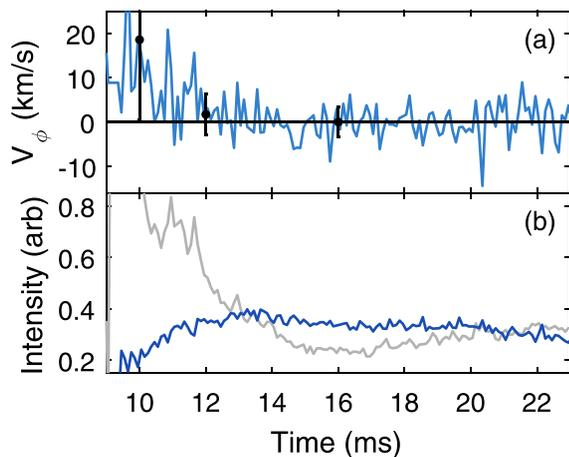
FIG. 3. Zero-flow calibration shot at  $r=0$  cm. (a) Calibrated poloidal velocity. The three error bars represent the measurement noise at three characteristic time points. (b) The intensities of the active charge exchange signal (dark blue) and the background signal (light gray) as functions of time.
