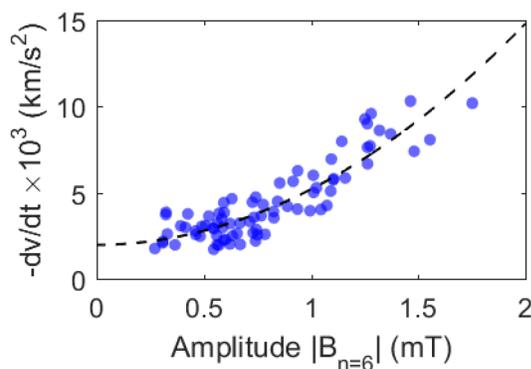
**FIG. 10.** Correlation between the  $n=6$  mode deceleration and  $n=6$  mode amplitude. A quadratic model gives the best fit.
