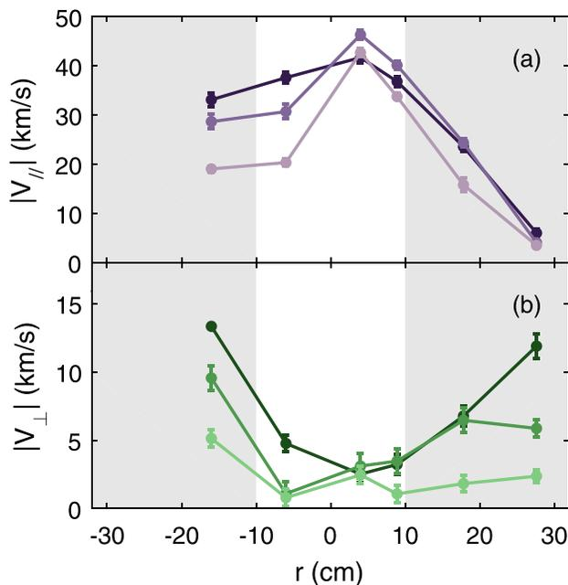
**FIG. 5.** (a) Parallel and (b) perpendicular flow profiles calculated from average poloidal and toroidal flows in Fig. 4. Profile lines evolve from darkest to lightest tone, with time windows 12–14 ms, 15–17 ms, and 18–20 ms. Error bars represent the variation in the data from individual discharges. The shaded regions indicate the regions where tearing modes are resonant.
