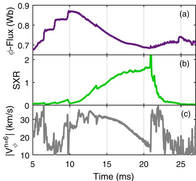
FIG. 1. (a) Toroidal magnetic flux, (b) soft X-ray emission (arbitrary units), and (c)  $m = 1$ ,  $n = 6$  toroidal phase velocity are shown for a typical PPCD discharge. PPCD is active from 10 ms to 20 ms.
