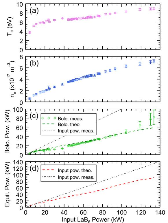
FIG. 8. The scaling of (a)  $T_e$ , (b)  $n_e$ , and (c) radiated power measured while varying the input power from 4 to 135 kW into  $6.5 \times 10^{-5}$  Torr helium. The data are used to predict the radiated and equilibrium power required using a confinement a model, which is compared to the input power (d) by the LaB<sub>6</sub> cathodes.
