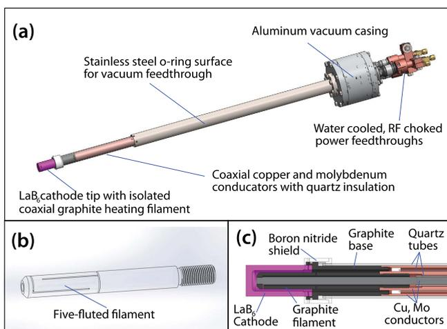
FIG. 4. LaB<sub>6</sub> stirring electrode design. The entire (1.1 m long) electrode is shown in (a), with detailed views of (b) the graphite heater filament and (c) the LaB<sub>6</sub> tip. Not shown: the linear vacuum feedthrough and garage/gate-valve assembly.
