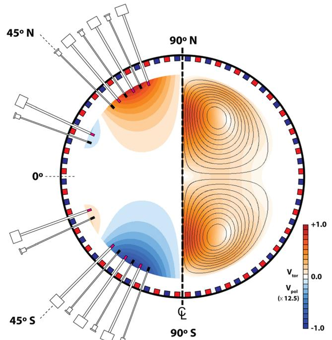
FIG. 13. Numerical simulations of the boundary driven flow for the flow drive with  $Re = 300$  in a Von Kármán geometry with counter rotating flows in each hemisphere. The poloidal flows (right side) develop self-consistently as a response to the centrifugal forces developing due to toroidal (left) rotation.
