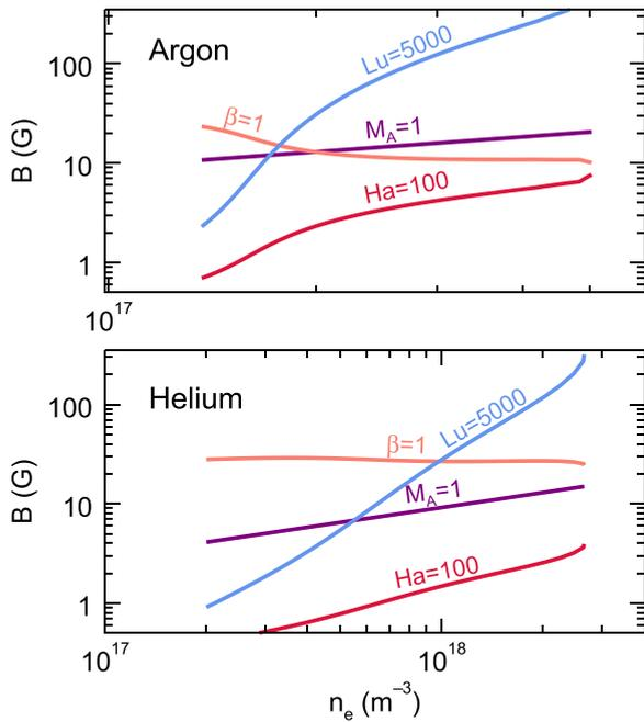
FIG. 12. The threshold magnetic field (G) for various astrophysically relevant dimensionless magnetic scaling parameters for (a) argon and (b) helium, the Alfvén Mach numbers  $M_A = 1$ , the Lundquist number  $S = 5000$ , and the Hartmann number  $Ha = 100$ . These values are predicted using the confinement code for a 300 kW discharge for  $v_\phi = 10$  km/s and  $1 \text{ G} < B < 100 \text{ G}$ .
