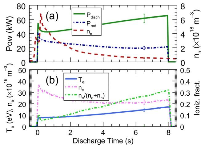
FIG. 6. (a) Time trace of the gas puff, the input power, and the radiated power from the bolometer (b)  $T_e$  measured by a Langmuir probe,  $n_e$  measured by an interferometer normalized to a path length measured by probes, and the calculated ionization fraction  $n_e/(n_n + n_e)$ .
