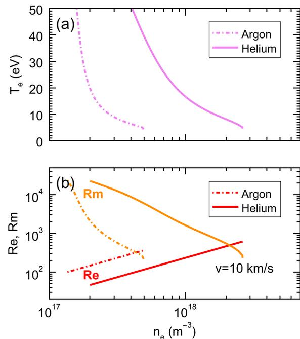
FIG. 11. Plasma parameters calculated using the confinement code described above for an input power of 300 kW and  $v_\phi = 10 \text{ km/s}$  over a scaling of  $n_e$  achieved by varying the fill pressure in argon (dashed) and helium (solid). (a) The tradeoff between  $T_e$  and  $n_e$ . (b) The tradeoff between  $Re$  (red) and  $Rm$  (orange). This creates a scaling of magnetic Prandtl number  $0.01 < Pm = Rm/Re < 100$  with the intersections of the lines corresponding to  $Pm = 1$ .
