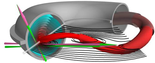
FIG. 3. SHAx plasma with both CHERS optical views (toroidal and poloidal) and neutral beam (gray). The two light cones (green and purple) represent the off-beam and on-beam views respectively for both poloidal and toroidal CHERS views. The black lines show the intersection of representative flux surfaces obtained by V3FIT with the plane that would be sampled by the neutral beam as the plasma is rotated through the beam.
