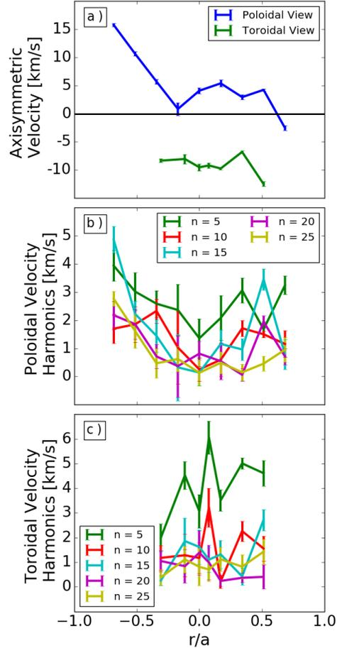
FIG. 6. a) Axisymmetric ( $n=0$ ) poloidal (blue) and toroidal (green) flow profiles. b) Poloidal and c) toroidal harmonic flow profiles. Error bars represent the standard deviation of the velocity amplitudes from fitting ten random subsets of the total dataset.
