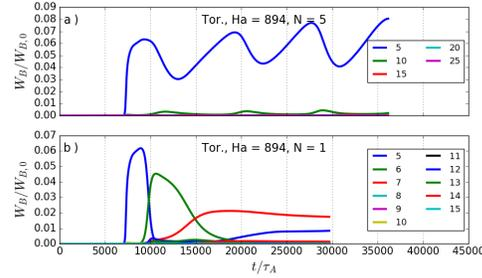
FIG. 12. Time evolution of the total magnetic mode energy,  $W_B$ , normalized by the total axisymmetric magnetic energy,  $W_{B,0}$ , high dissipation ( $Ha = 894$ ) NIMROD simulations in toroidal geometry for a)  $1/5$  of a torus ( $N = 5$  limited periodicity boundary condition) and b) the entire torus ( $N = 1$  periodic boundary condition). The  $n = 5$  mode dominates over higher  $n$  modes, but in a) the mode oscillates strongly and in b) other modes rise up to become dominant.
