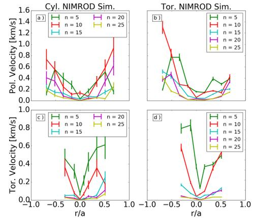
FIG. 11. Average NIMROD velocity mode amplitudes from the time points shown in the dotted black lines in Figure 7 at the same radial locations and orientations as the CHERS diagnostic in MST. Poloidal and toroidal flow is provided in a) and c) respectively for the cylindrical geometry simulation and b) and d) respectively for the toroidal geometry simulation. Error bars represent the standard deviation of velocity amplitude used in the averages.
