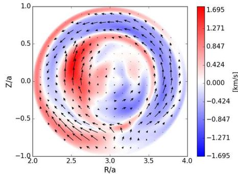
FIG. 10. Poloidal cross-section of the toroidal geometry NIMROD simulation showing velocity at  $5\phi_{\text{SHAX}} = 1.5$  rad and time point  $t/\tau_A = 18069$ . The black arrows show the direction of velocity in the poloidal plane, with the length of the arrow representing the relative strength of the flow, and the color scale represents the toroidal velocity.
