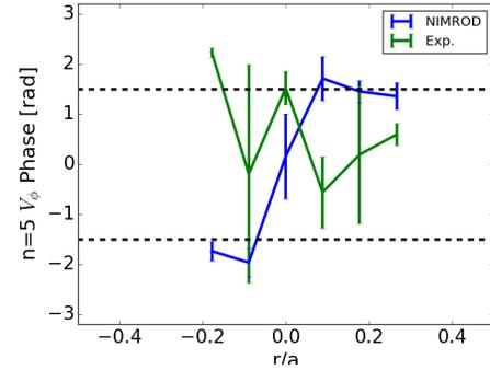
FIG. 14. Phase of the helical flow for the experimental data (green) and the toroidal NIMROD simulation (blue). A phase of  $\pm\pi/2$  indicates the flow extremum is out-of-phase with the helical magnetic axis, as would be predicted from single-fluid MHD. A phase shift away from  $\pm\pi/2$  is indicative of a decoupling of the ion and electron fluid.
