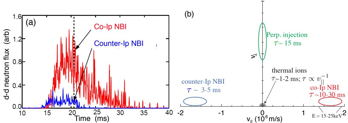
**FIGURE 2.** (a) NBI-sourced test ions show a confinement asymmetry. In red (blue), 25 keV D+ ions injected parallel (anti-parallel) to plasma current produce fusion neutron flux with different decay timescales. (b) Illustration of known ion confinement behavior as a function of position in  $v_{\perp}/v_{\parallel}$  plane. A boundary between thermal and highly energetic ions must exist.
