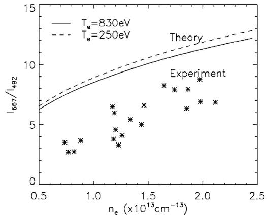
FIG. 3. Dependence of  $I_{667}/I_{492}$  on the local electron density. The theoretical line ratio was calculated for the upper and lower bounds of the experimentally measured  $T_e$  values. The theoretically anticipated insensitivity of the ratio to the electron temperature could not be confirmed due to the lack of experimental data.
