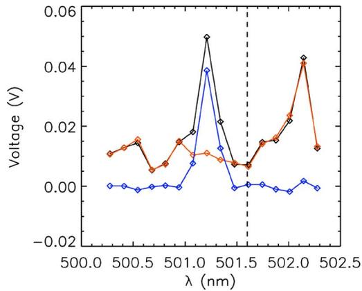
FIG. 2. (Color online) Doppler shifted 501.6 nm He I beam emission line; net beam contribution is represented by the blue line, which is the result when the background channel (red) is subtracted from the beam channel (black). The vertical line represents the wavelength of the non-Doppler shifted 501.6 nm He I line.
